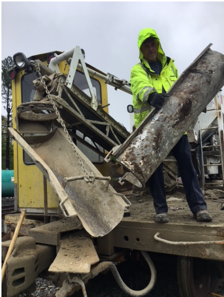
Photo 4- Second Section of Chute Damaged
