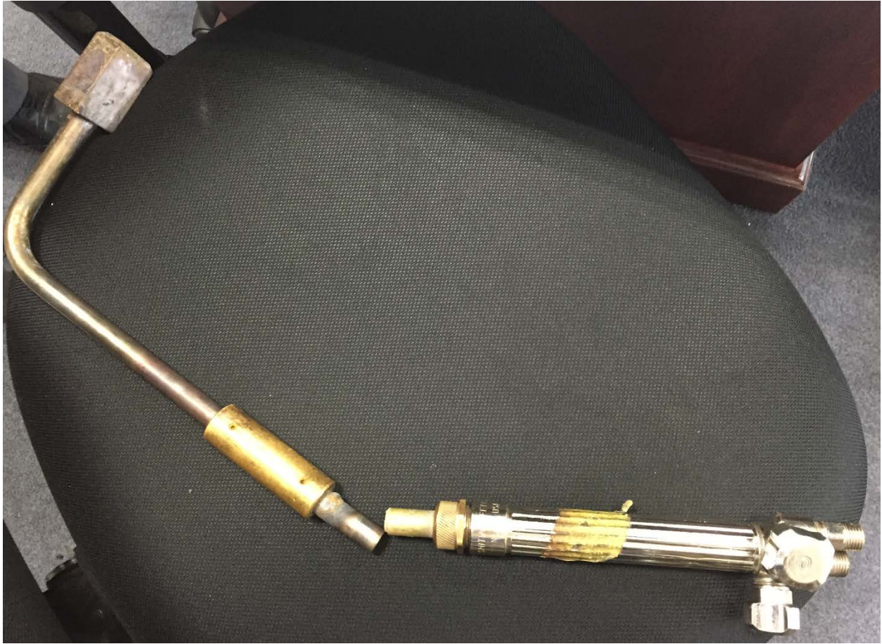
Photo 3 – Broken torch which caused injury
