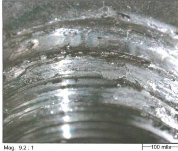
Figure 7: The nut threads were damaged in the same way as the bolt threads.
