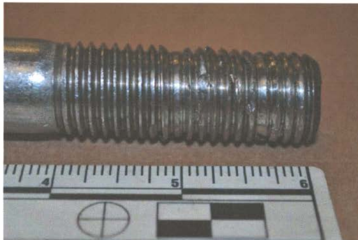
Figure 2: Overall view of thread damage on the submitted bolt.
