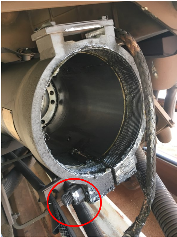
Photo 5 – Car 6038 Buffer Tube Screw torque strip moved
