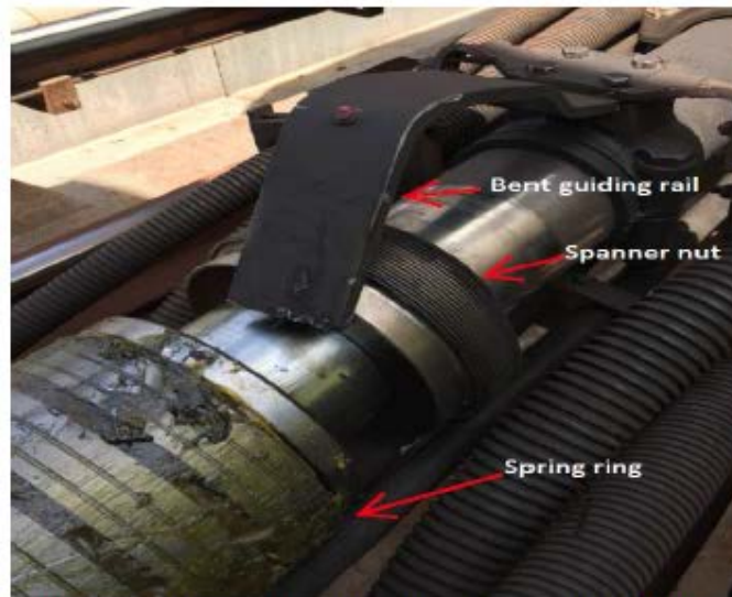
Figure 3 – Bent guiding rail and Ring spring (Car 6039)
