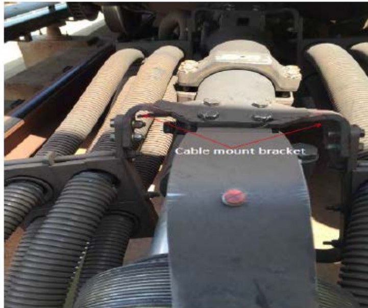
Figure 4 – Damaged Upper cable mount bracket (Car 6039)
