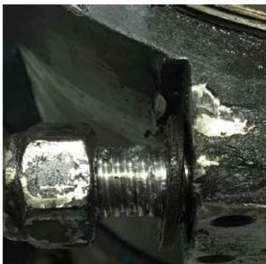
Figure 11a – Cross Threaded Buffer tube lock Screw
