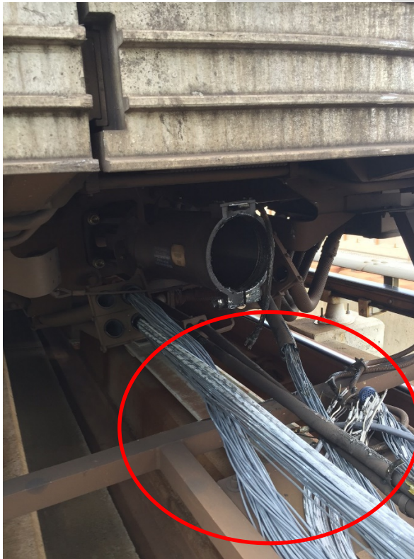
Photo 4 – Car 6038 Trainline Wiring Damage
