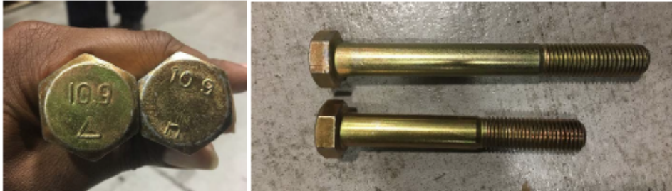
Figure 13 – Incorrect Zinc Plated bolts. Found in stock room under C18-36-6091 (& C18-36-6051)
