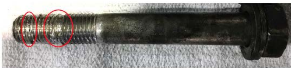
Figure 11b – Cross Threaded Buffer tube lock Screw
