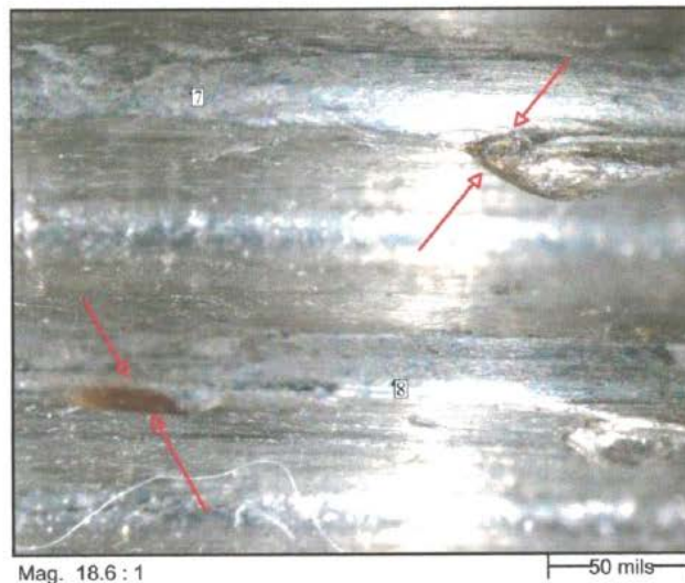
Figure 6: Heat tint on threads 7 and 8, arrows.
