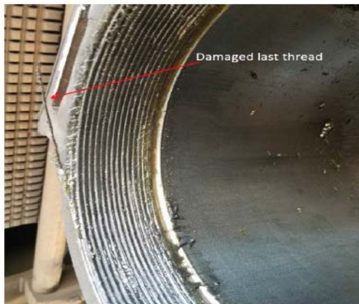
Figure 5 – Only last thread was damaged on Buffer tube (Car 6038)
