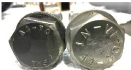
Incorrect A4-70 screw Correct A4-80 screw Figure 12 – A4-70 and A4-80 Locking Screws Page 11 of 13
