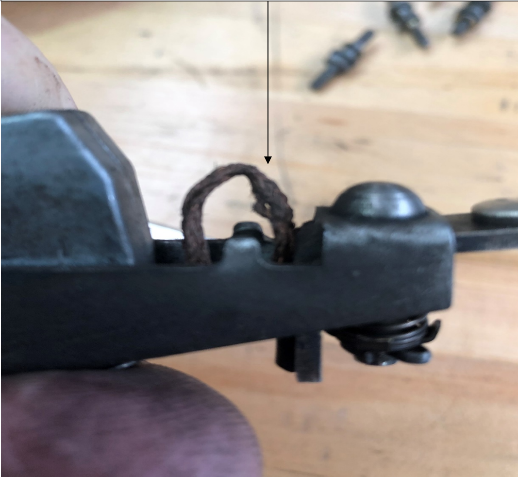
Photo 3 – Significant finding, shunt damage
