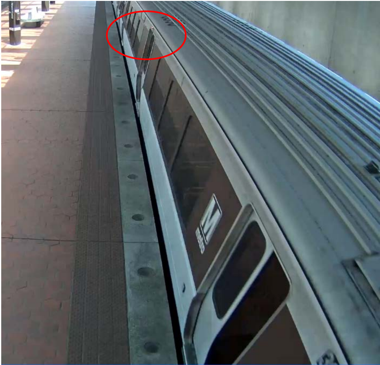
Photo 12 – 13:55:20 door indication lights illuminated while train in motion
