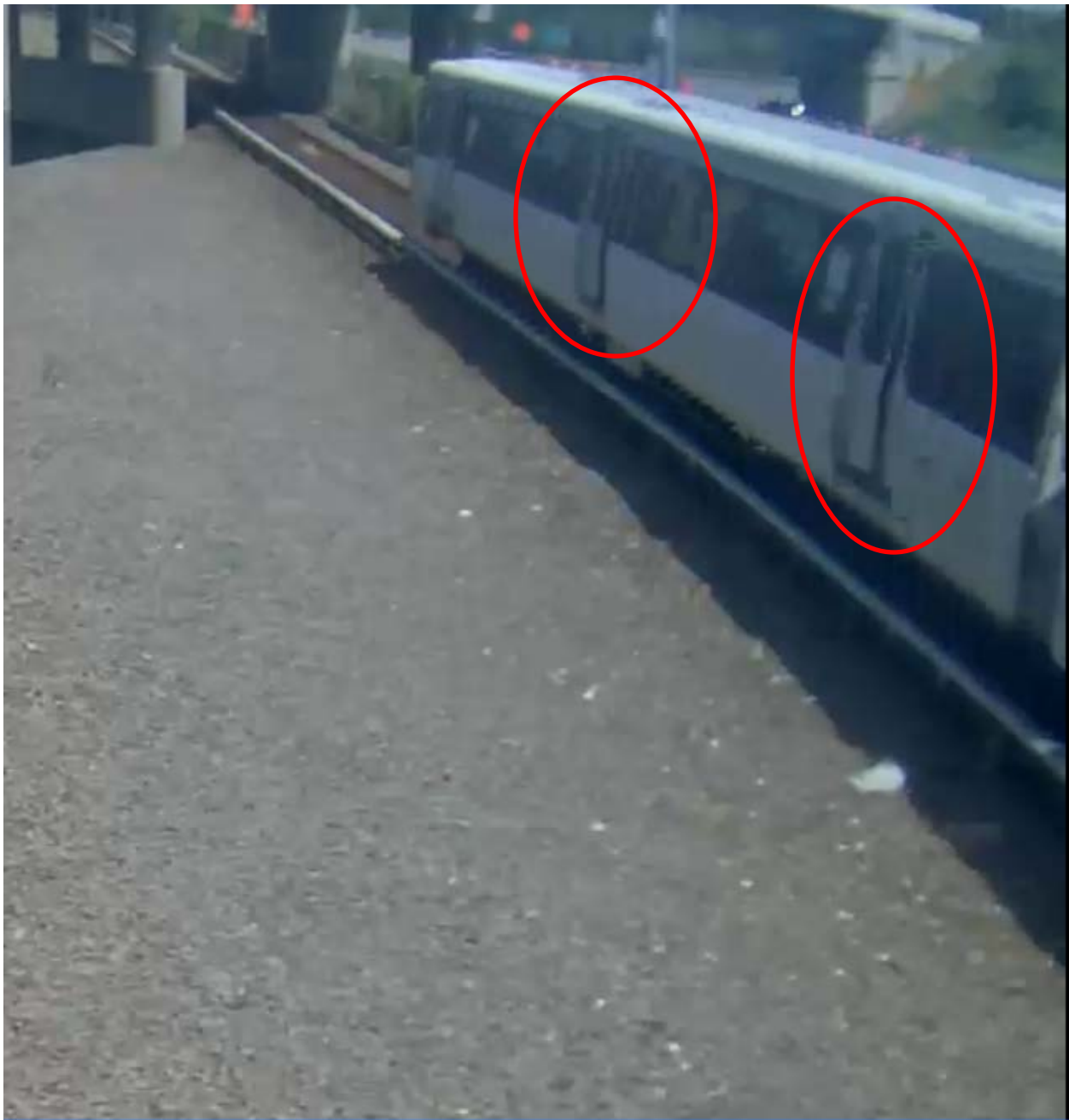
Photo 11 – 13:55:20 doors began to close while inertia prevents right leaves from closing.
