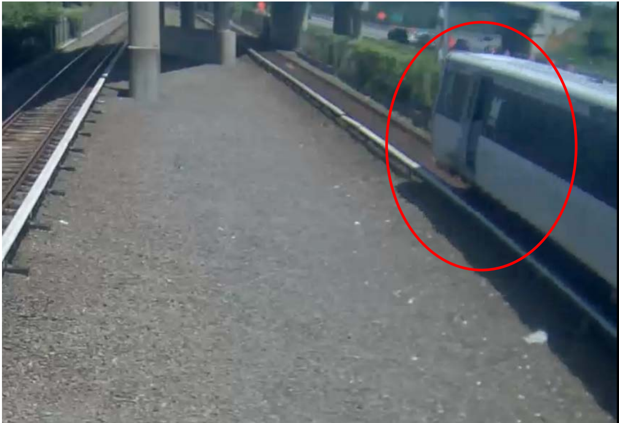
Photo 10 – 13:55:19 Doors open while train in motion outside platform limits
