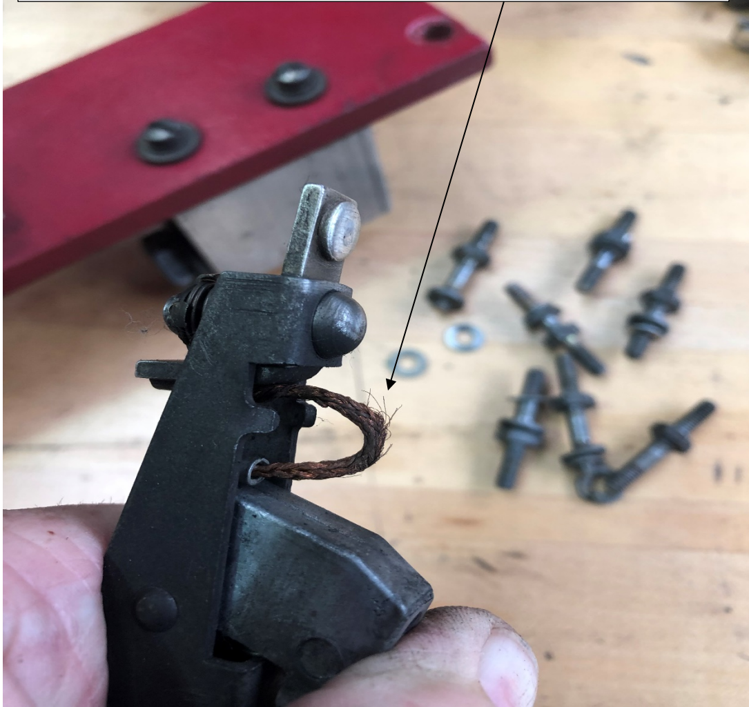
Photo 7 - Minor Finding, shunt with Damage
