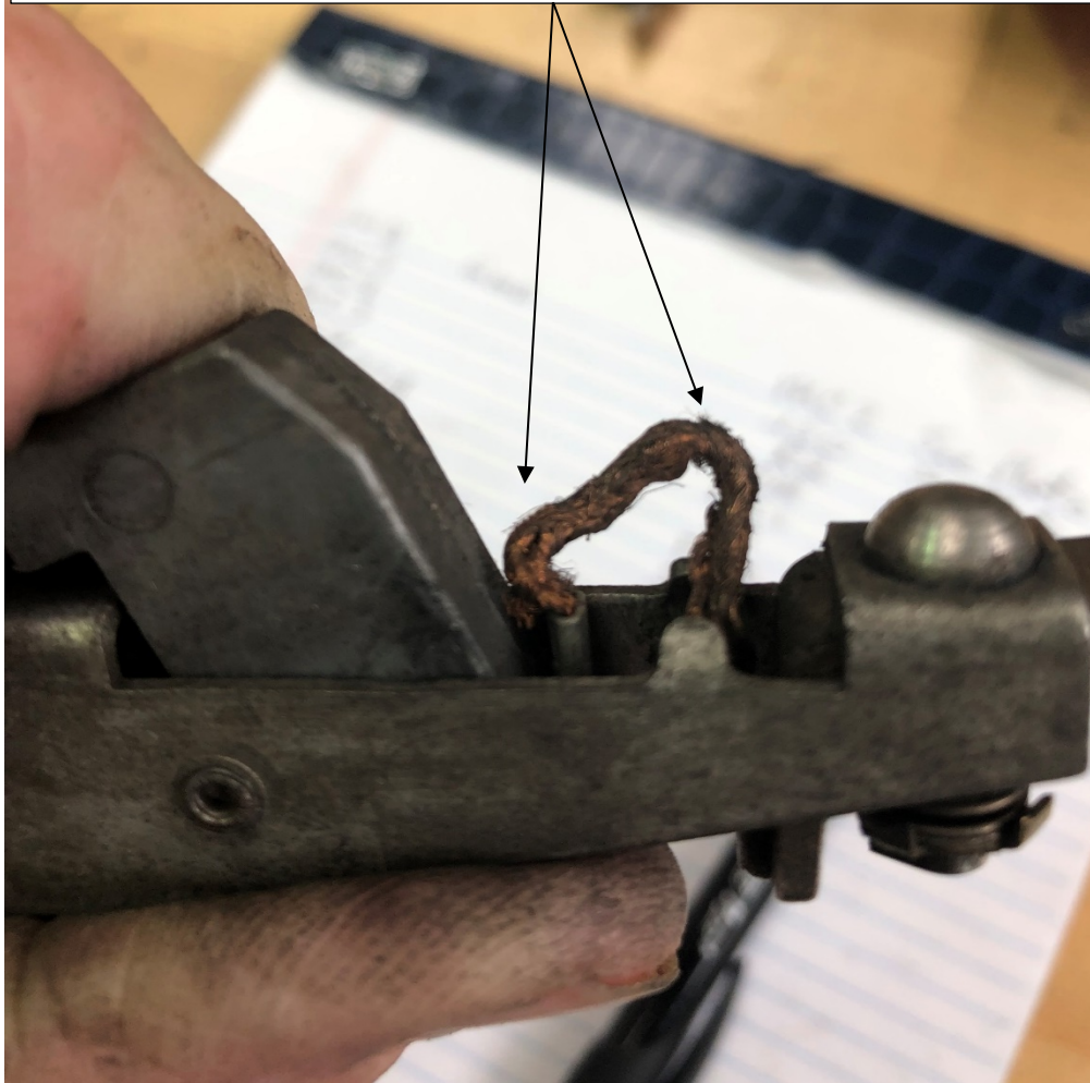
Photo 6 - Minor Finding, shunt with Damage
