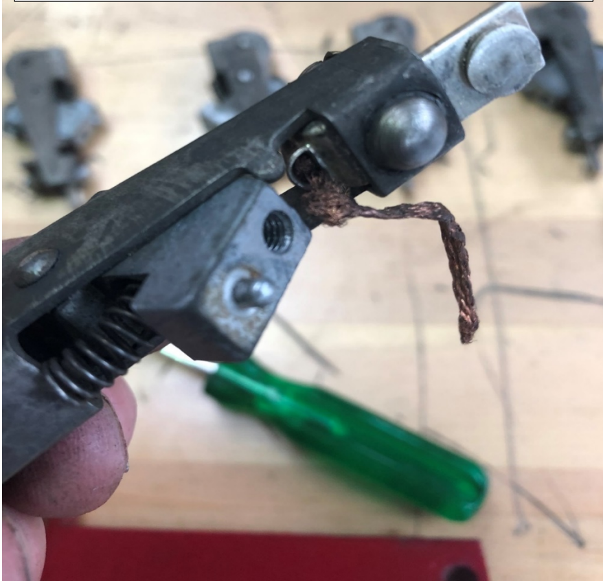
Photo 1 - Major Finding / Root Cause of Door event involving Car 3135
