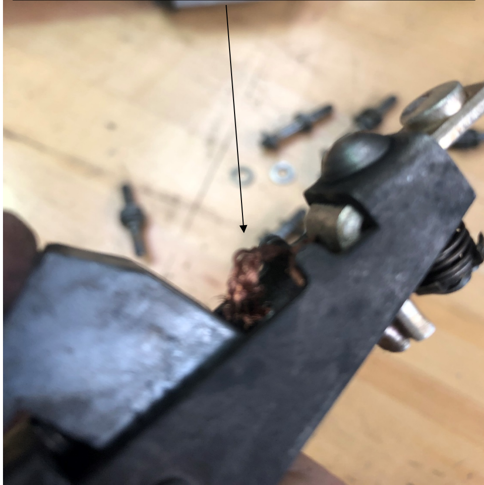
Photo 5 – Significant finding, shunt damage
