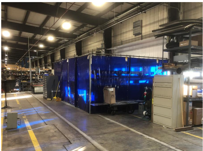
Photo 4 – A missing curtain barrier from the hot works area was installed
