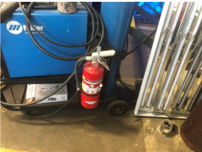
Photos 6 and 7 – Fire extinguisher inspection labels were missing from some fire extinguishers
