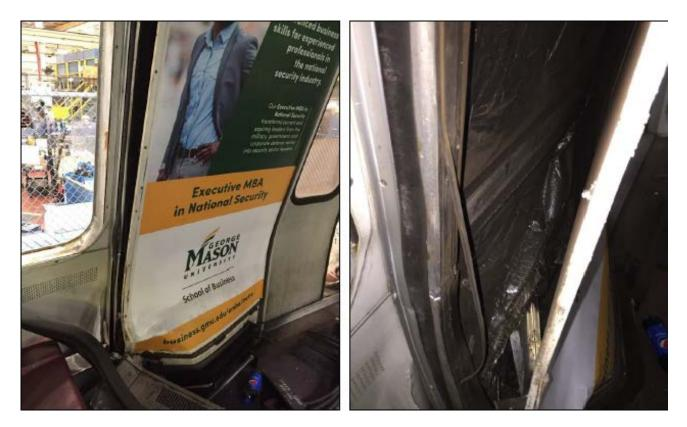
Photo 9 and 10 – October 09, 2019, Car 3008 – Photos showing damaged door pocket and décor panels.
