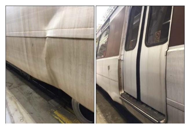
Photo 17 and 18 – October 09, 2019, Car 3009 – Photo showing exterior body panels buckled.
