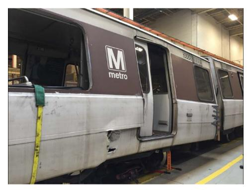
Photo 16 – October 09, 2019, Car 3008 – Photo showing exterior body panels buckled.
