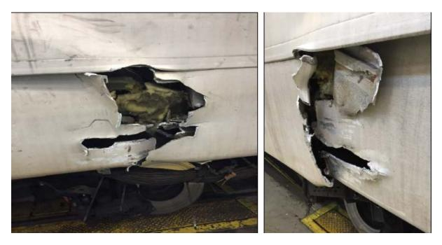
Photo 14 and 15 – October 09, 2019, Car 3008 – Photo showing exterior body panels buckled.
