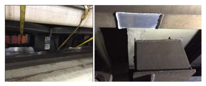
Photo 7 and 8 – October 09, 2019, Car 3008 – Photo showing broken Propulsion Common Case brackets.
