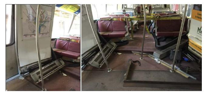
Photo 11 and 12 – October 09, 2019, Car 3008 – Damaged floor heat covers, stanchions, floor and décor panels.
