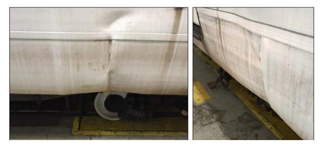
Photo 19 and 20 – October 09, 2019, Car 3206 – Photo showing exterior body panels buckled.
