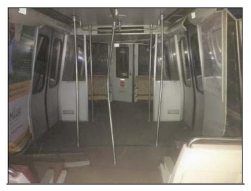
Photo 1 – October 07, 2019, Car 3008 – Photo showing floor, stanchions and side décor panels buckled.
