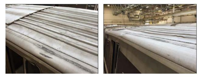
Photo 5 and 6 – October 09, 2019, Car 3008 – Photo showing roof buckled and sings of roof making contact with tunnel ceiling.
