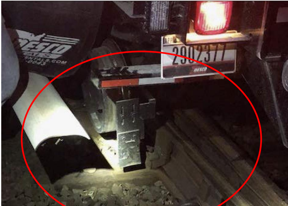
Photo 1 – Left Rear of HRU Wheel Derailed
