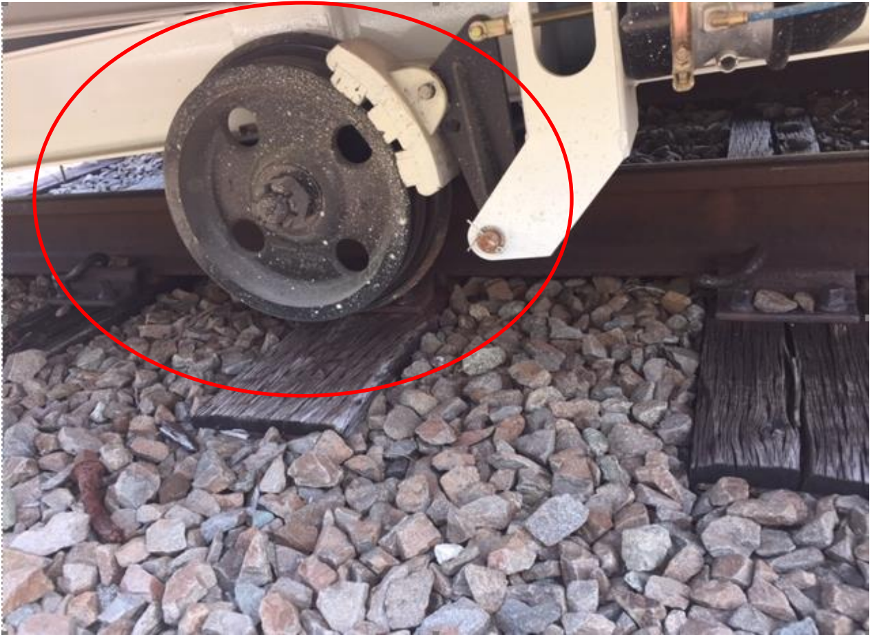
Photo 1 – Rear axle derailed on the field side
