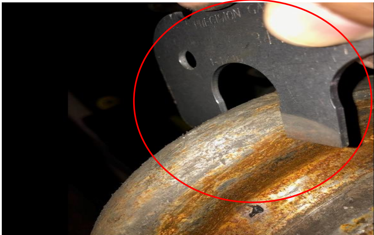
Photo 5 – SRS HRU Inspection includes inspection of the hi-rail wheels to validate they are within specification with a Caliper
