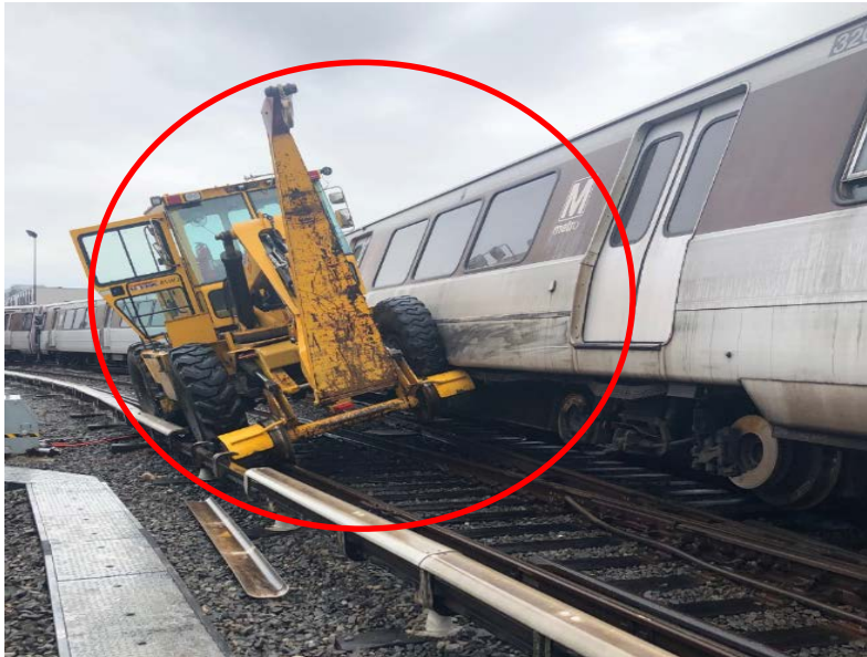
Photo 2 - This collision resulted in both vehicles' wheels losing contact with the rails.
