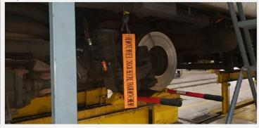
Cars 3122-3 were located at station one on the 9-north track. At the time of inspection there was no active work being performed. On rail car 3123, the bulkhead door was inspected and an issue with the door seal was found and discussed with the WMATA escort. One axel was chalked with a warning flag present and track nine was blue flagged.
