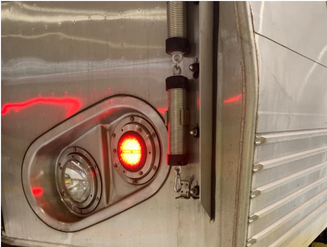
Photo 3 - Inter-car barriers were in the stowed position, but they were not engaged
