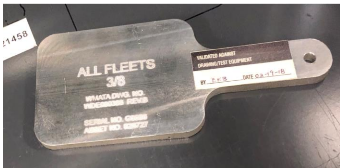
Photo 5 – Special tool was overdue for calibration
