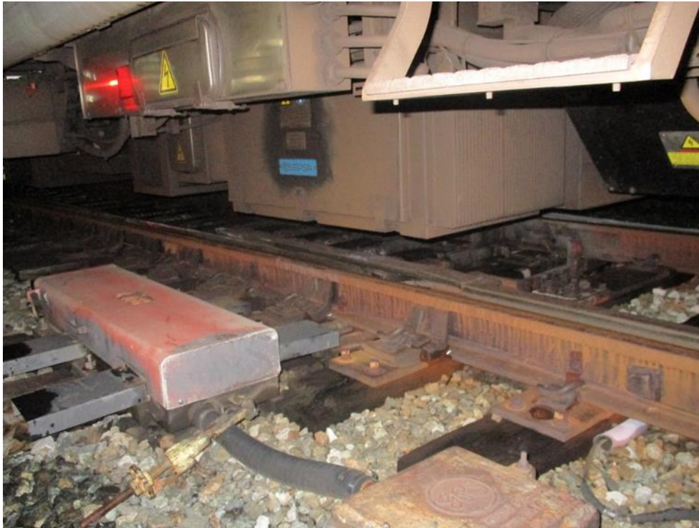
Photo 5: Incident train traveled through Switch 141B after passing Signal B99-138 (Red), Track #1.
