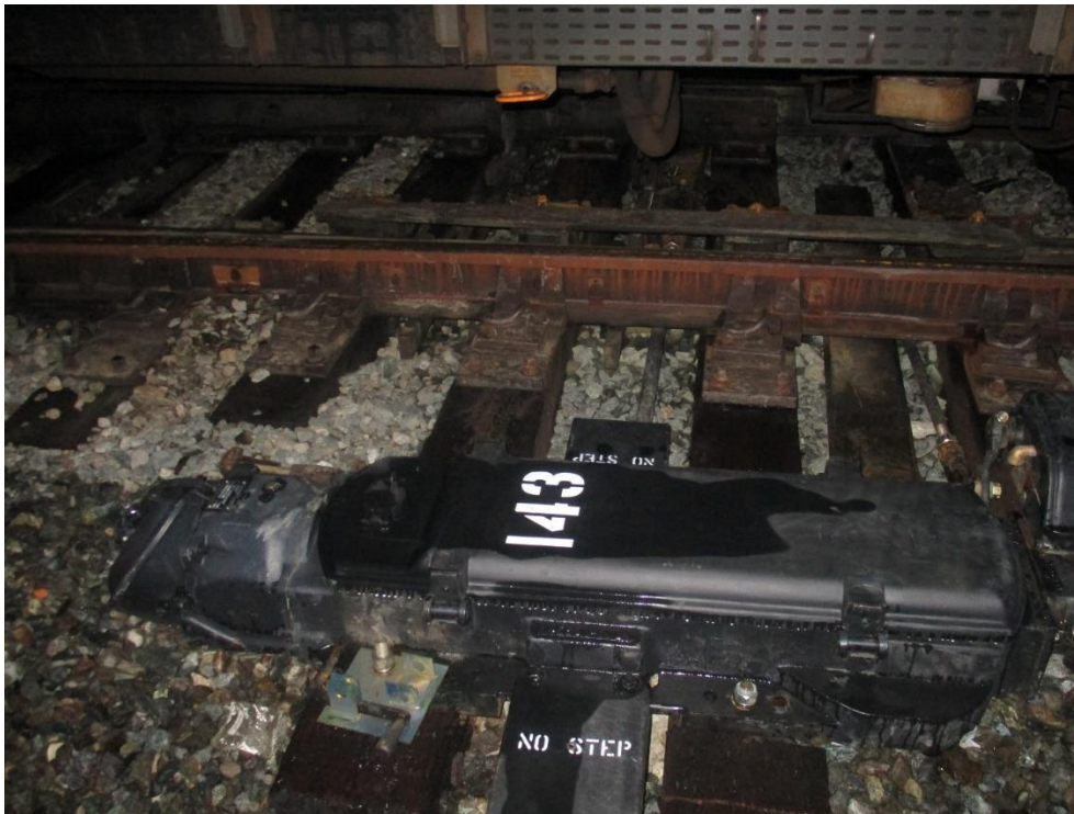
Photo 6: Incident train traveled through Switch 143 after passing Signal B99-138 (Red), Track #1.
