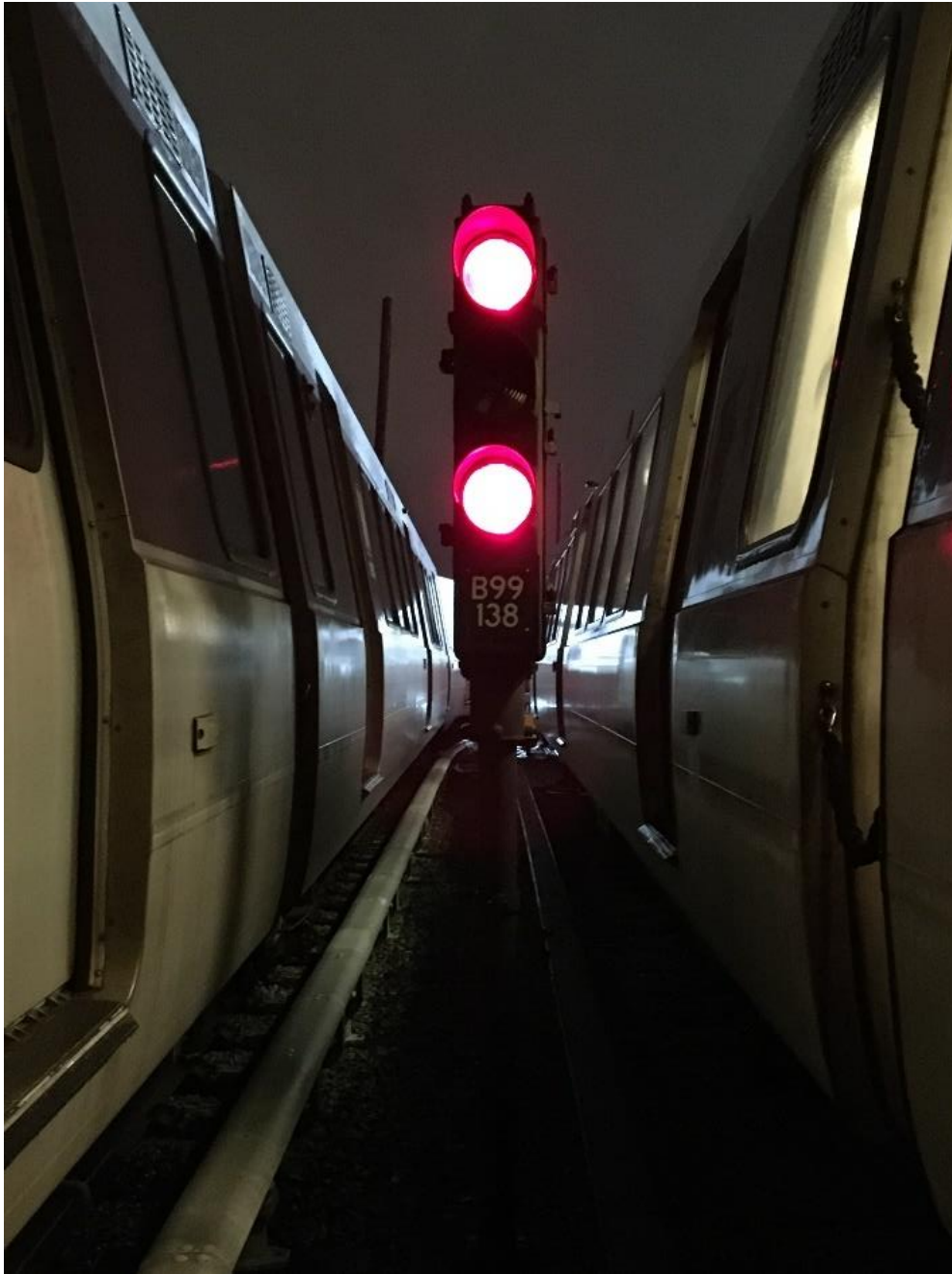
Photo 9: Signal B99-138, Track #1. Incident consist (left) stationary 231 feet past signal.
