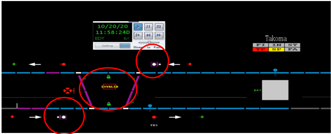
Diagram 2: AIMS displaying the interlocking in an “Invalid” state indicating the control key has been turned, allowing for ROCC to take control.
