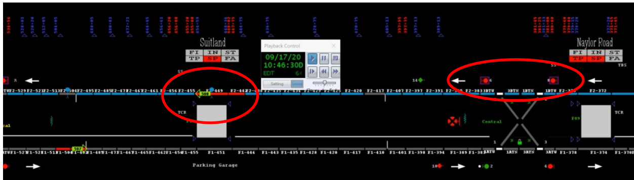
Photo 1: AIMS display indicating FT RWP for TRST at 10:46 hrs. Prohibit exits and red signals in place at F06-06 and F08-08 signals. TRST instructed to notify the Radio RTC when Train ID 508 clears their location on the mainline.
