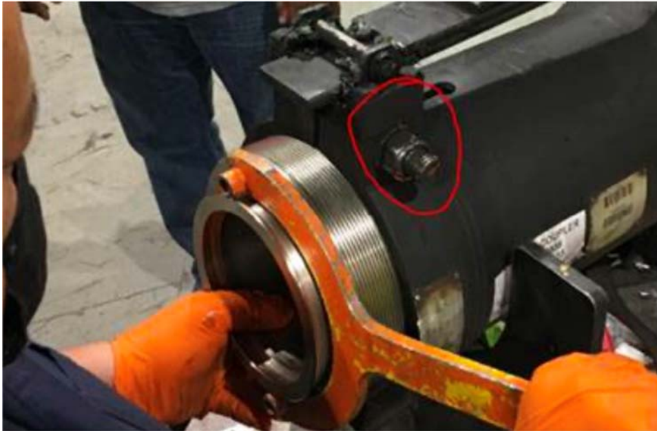
Figure 21: Actuation of gland nut with tightened bolt.
