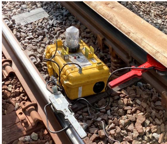
Figure 10: Locations and photo of the installed WSADs at the incident site.
