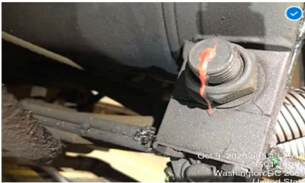
Figure 20: Torque mark on the same bolt pictured above prior to mechanical forces were applied.
