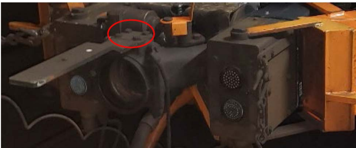
Figure 13 - A torque test was performed on the four guide rail bolts. The resulting torque was measured at 5 ft/lbs. Dellner documentation states torque should be 27 ft/lbs. The inspection of the coupler/drawbar revealed a lack of torque stripes on guide rail fasteners.
