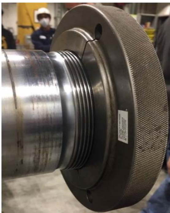
Figure 12 – While using the Dellner supplied Go/No-Go thread gauges on the draft bar threads, it was determined that the threads were worn. The draft bar must be condemned.
