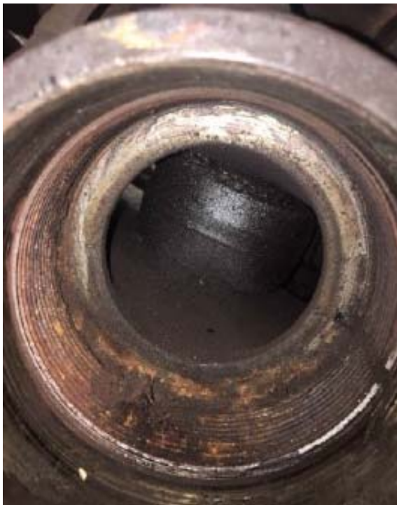
Figure 9: Corrosion and contaminants were found on the threads of the mechanical coupler head on car 6177.
