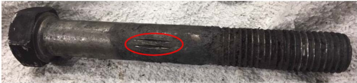
Figure 14 – A visual inspection revealed marks on the mechanical coupler head “pinch bolt” and identified that it did not have a torque stripe. Once removed, the bolt had two parallel indentations, which appear to have been caused by the threads of the draft bar.
