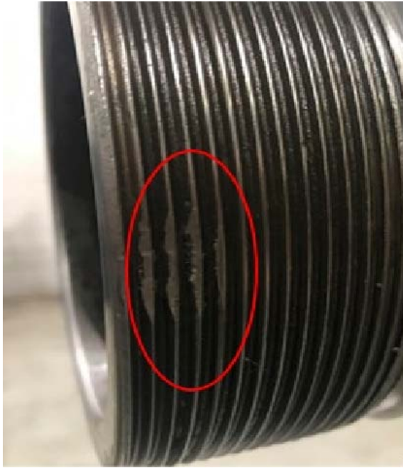
Figure 10: Damaged threads were found on the draft bar on car 6177.
