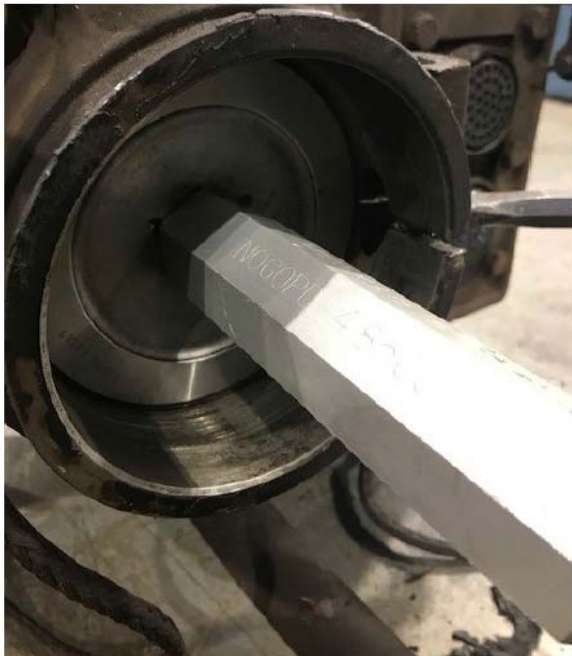
Figure 11 - While using the Dellner supplied Go/No-Go thread gauges on the mechanical coupler head threads, it was determined the threads were worn. The coupler head must be condemned.
