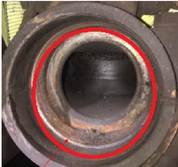
Figure 8: Corrosion and contaminants were found on the threads of the mechanical coupler head on car 6177.
