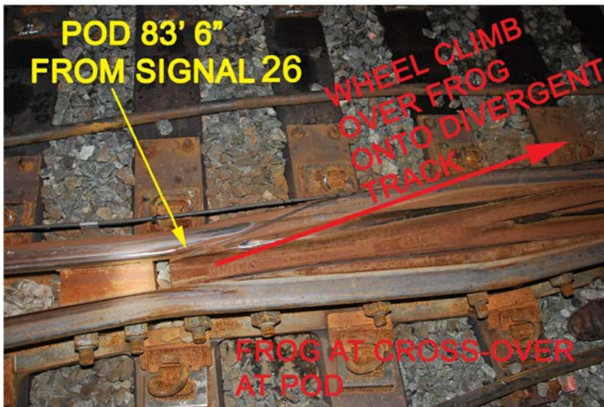
Photo 5 - Wheel climb marking of car derailed rear truck of car 7503
