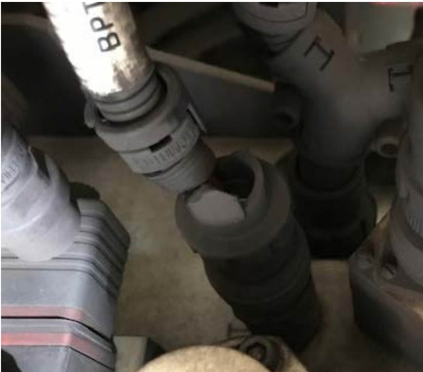
Car 7567 Broken plug at Front EPCU.
