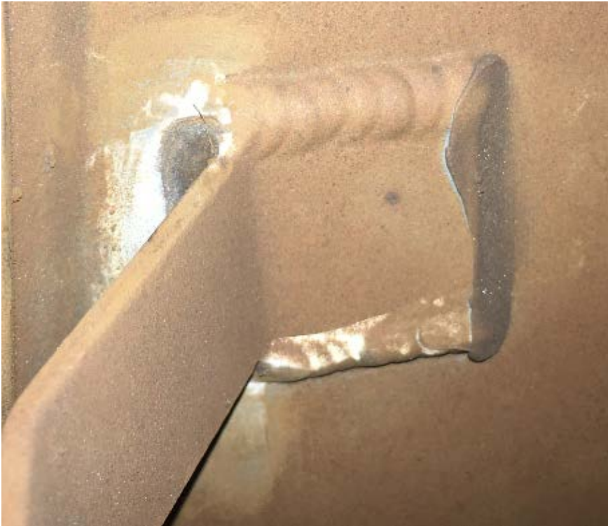
Car 7560: Hairline crack on pneumatic piping support bracket above wheel 1.
