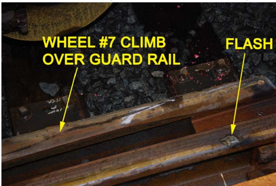
Photo 2 - POD wheel #7 climbed over the guard rail, and collector shoe contacted the running rail.
