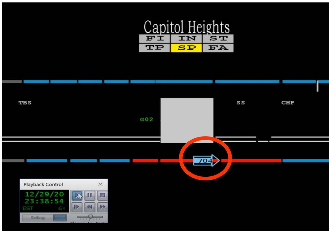
Diagram 2 - Based on the AIMS, at 23:38:54 hours, shows incident train's ID changed from 491 to 704.
