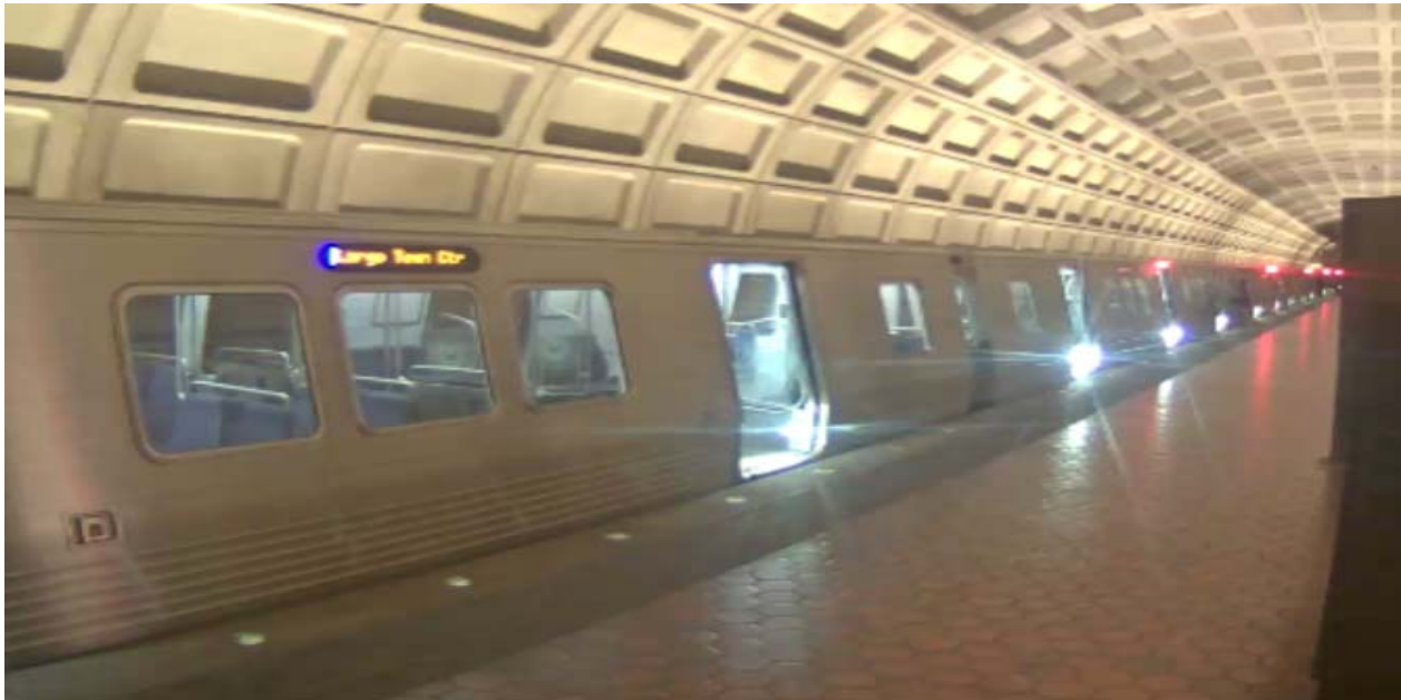
Figure 2 - Based on the CCTV, at 23:28 hours, the consist doors were commanded open on the opposite side of the Capitol Heights Station platform, Track 1.
