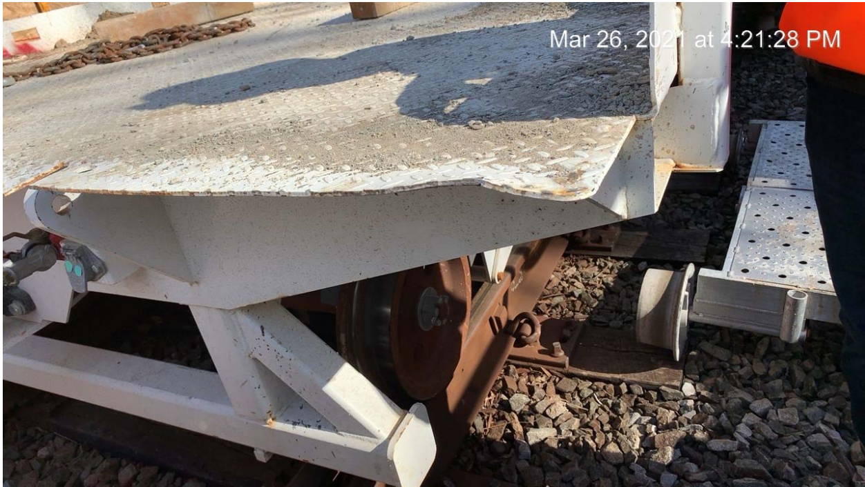
Photo 5: Damage to the tailgate as the result of the flatcar derailing. Total damages are currently pending.
