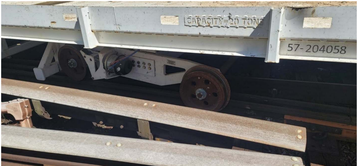
Photo 2: Wheel of flatcar derailed from the track.
