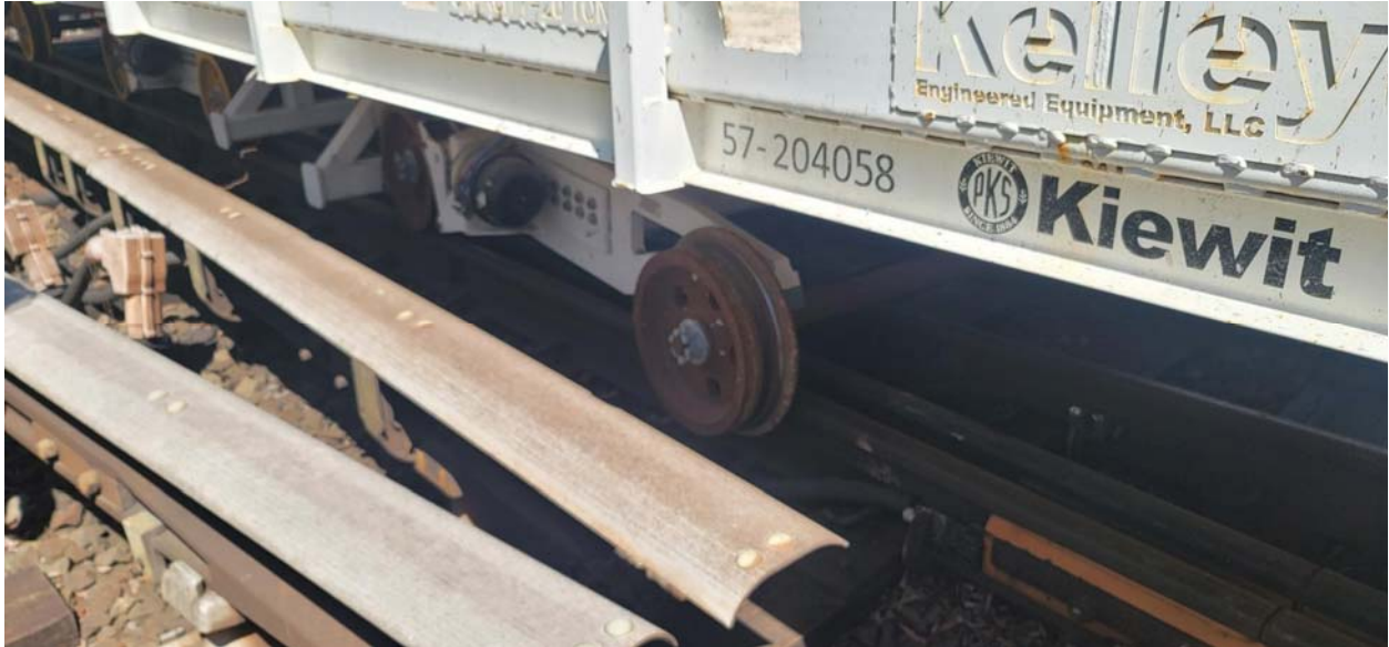
Photo 1: Wheel of flatcar derailed from the track.
