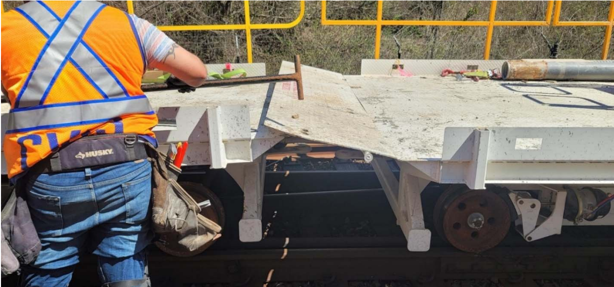
Photo 3: Flatcars with the tailgate down. Flatcar tailgates were in this position while traversing the switch from Track 2 to Track 1.
