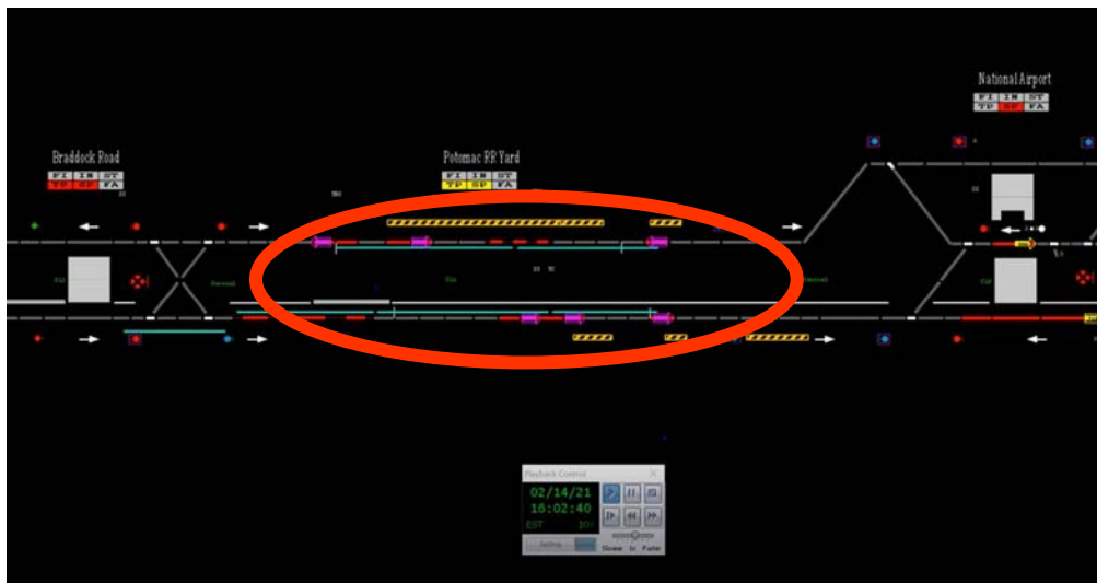
Diagram 3 - At 16:02 hours, the AIMS playback revealed, the power display indicated third rail power was de-energized at Potomac Yard Station, Track 1, and Track 2 before the fire department arriving on the scene and entering the roadway.
