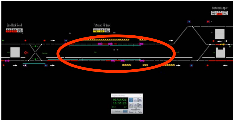
Diagram 4 - At 16:35 hours, the AIMS playback revealed that the power display indicated third rail power being de-energized at Potomac Yard Station, Track 1, and Track 2. AFD departed the scene and transported the Injured Contractor to Inova Alexandria Hospital for further medical evaluation.
