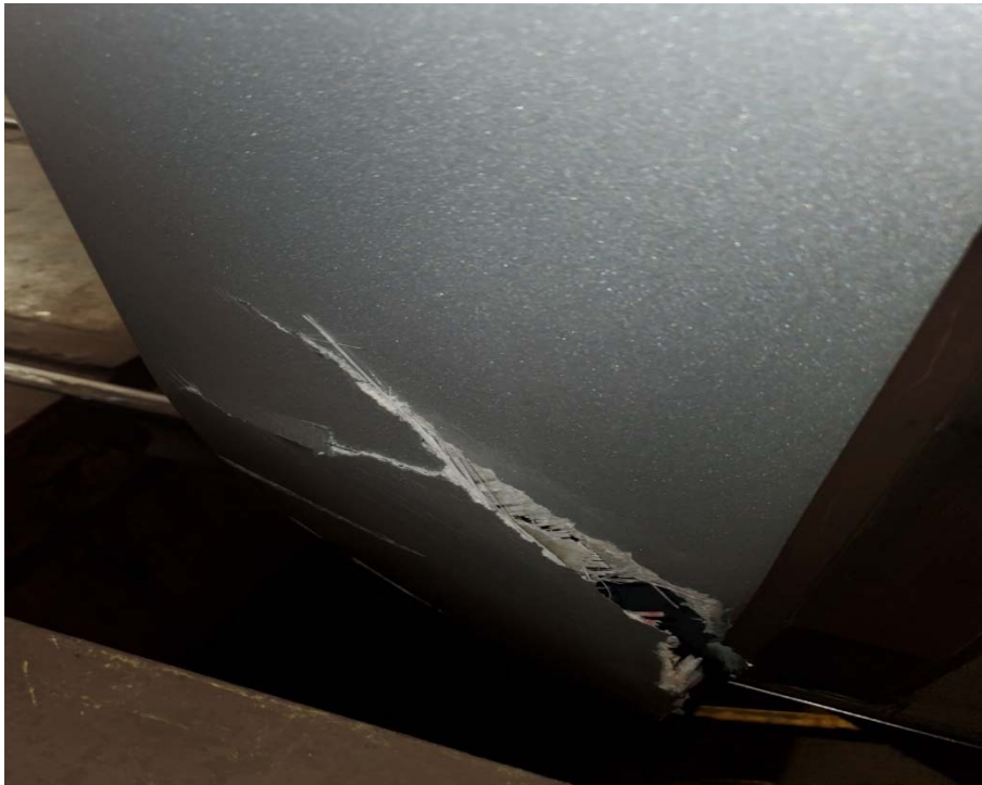
Photo 1 – Damaged sustained to the front cowling on lead car 7630.
