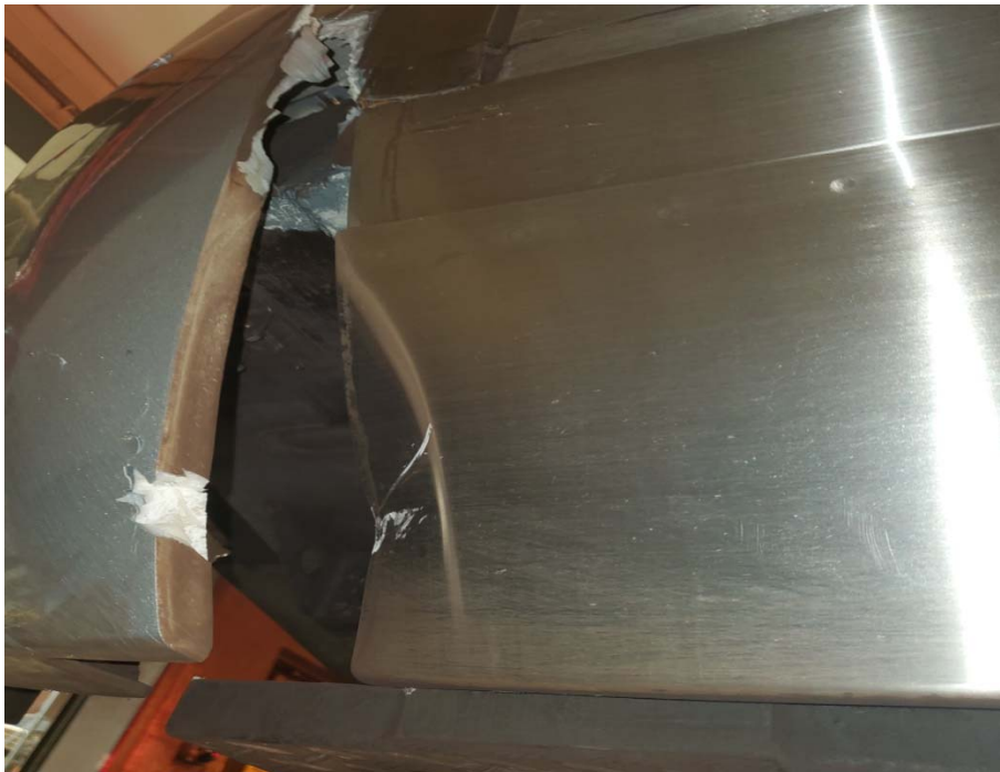
Photo 2 – Damaged sustained to the front cowling on lead car 7630.
