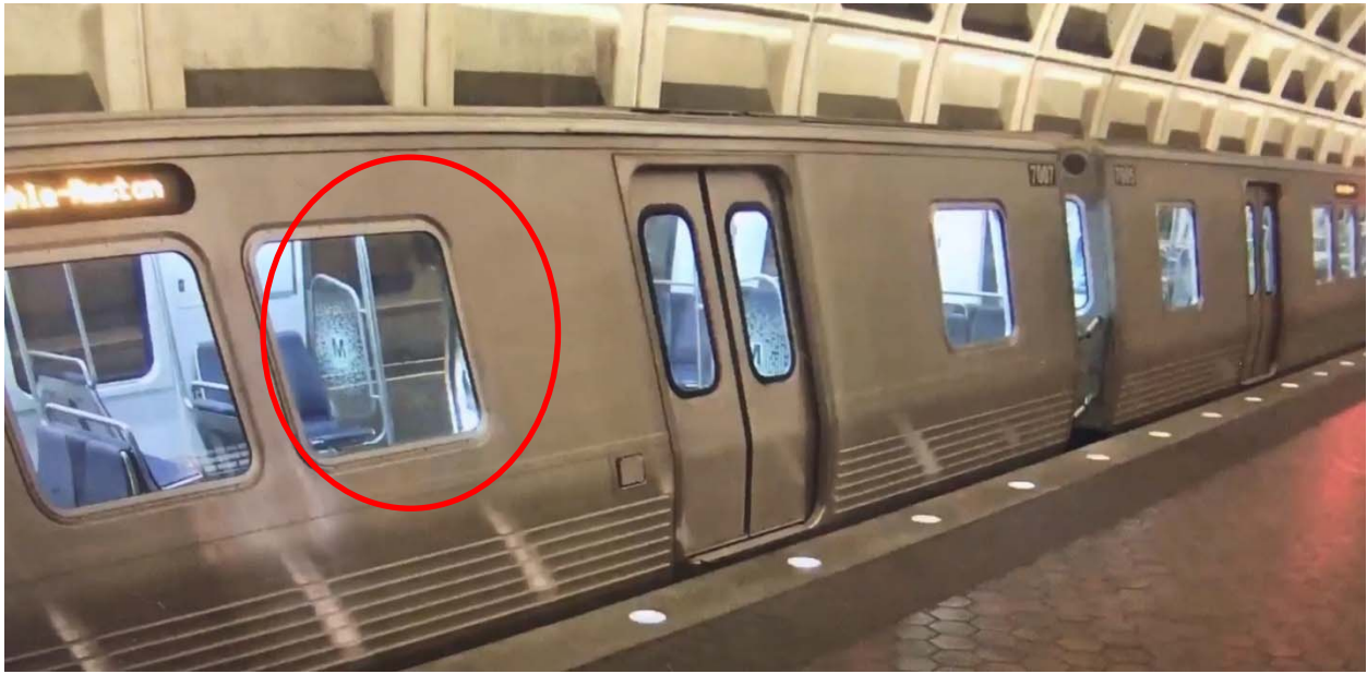
Photo #3 – Train ID 608 right side doors on the non-platform side completely opened.
