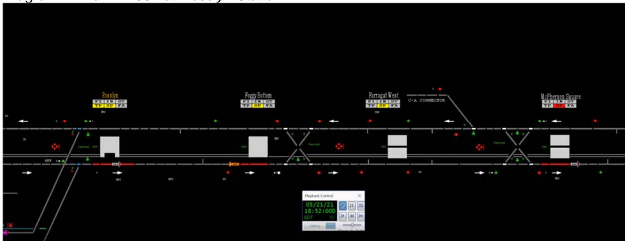
Diagram 2: Train ID 907 keyed up on the trailing end in Rosslyn Station's Direction
