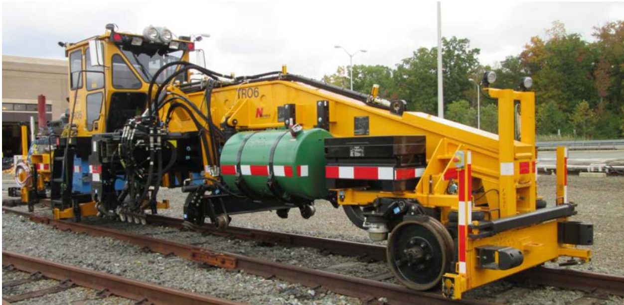
Figure 1 - TR06. This machine is a single-operator, climate-controlled, enclosed cab machine.
