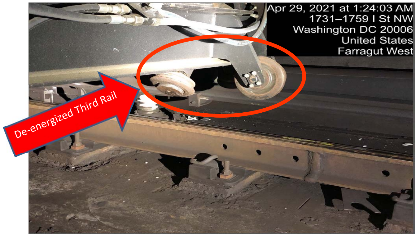
Figure 7 – TR06 rail clamp rollers, frame wheels derailed, and TR06 contacted the third rail.
