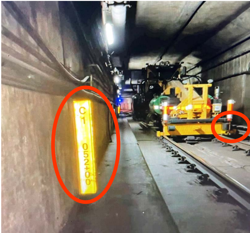
Figure 3 - TR06 derailed between CM C1-052+00 to CM C1-053+00 and made contact with the third rail.
