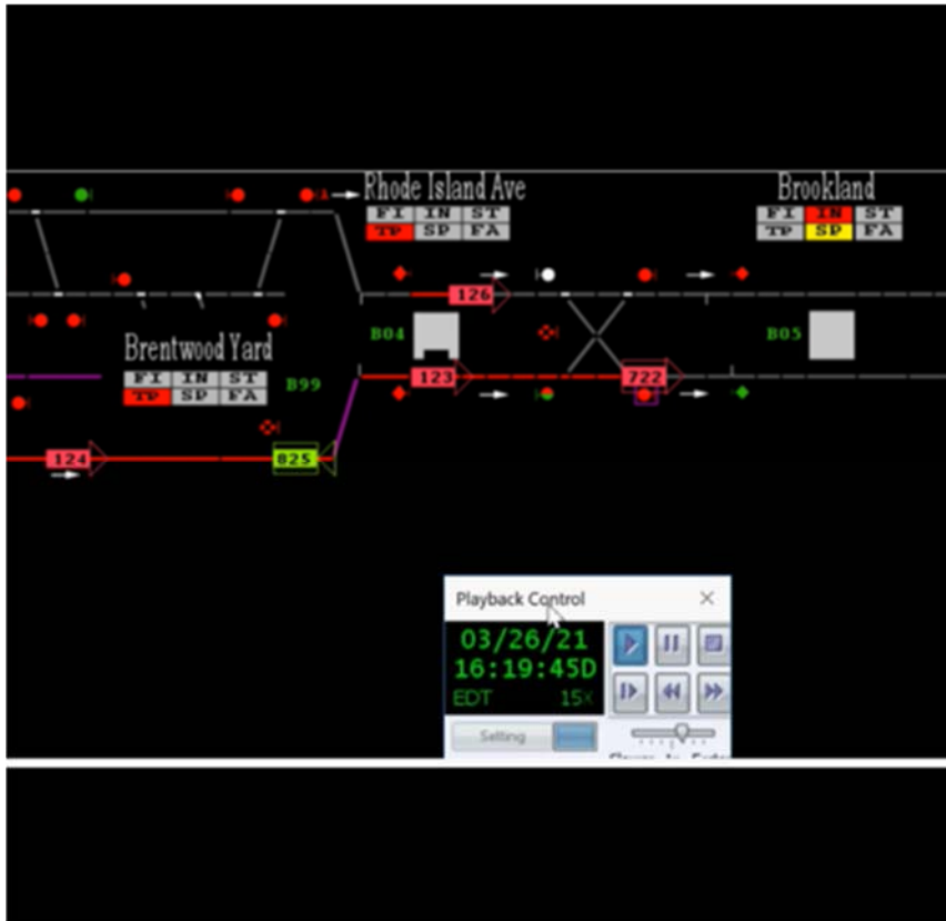
Diagram 3: Train ID 126 Departed Rhode Island Avenue Station after the customer was safely on the platform limits at Rhode Island Avenue Station.
