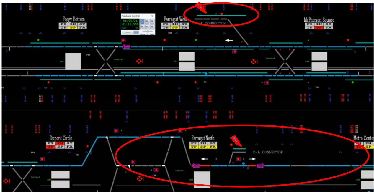
Diagram 2 (Ops 1) – Shows third rail power energized on the A-Line at 0126 hours; however, the C&A connector is de-energized
