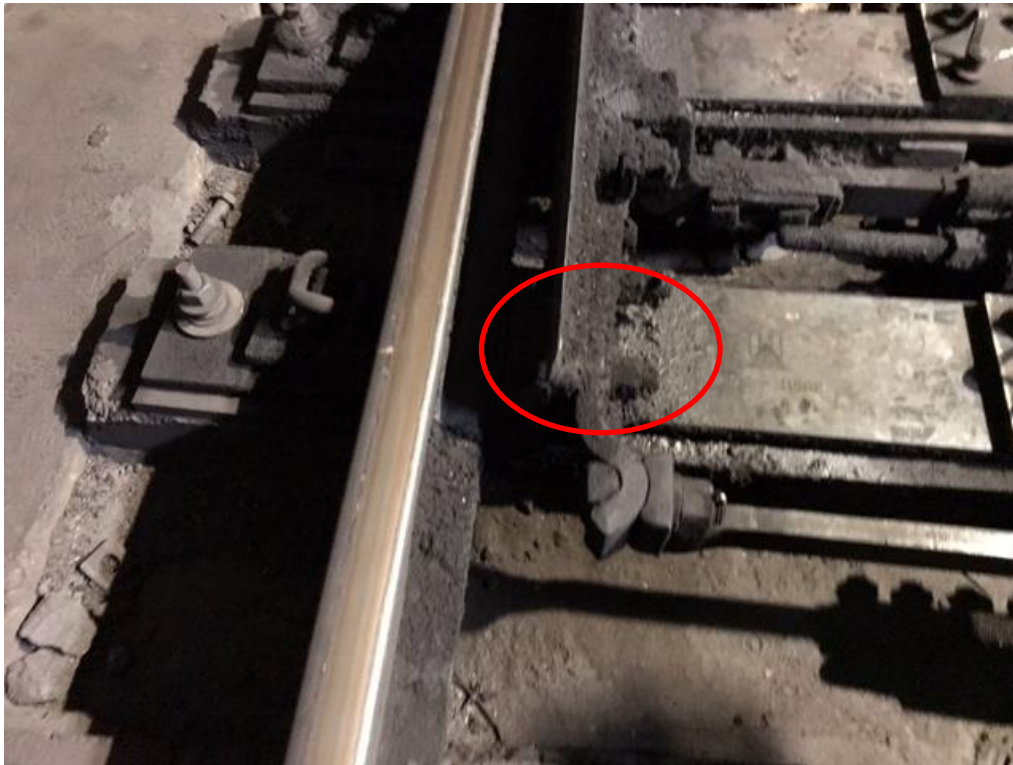
Photo 4 – Minor chip in the E03-08 switch point.
