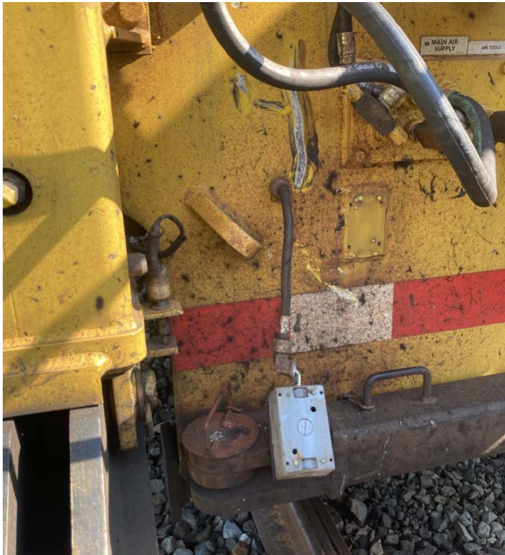
Figure 2 – Damaged electrical box on the left rear of PM65.
