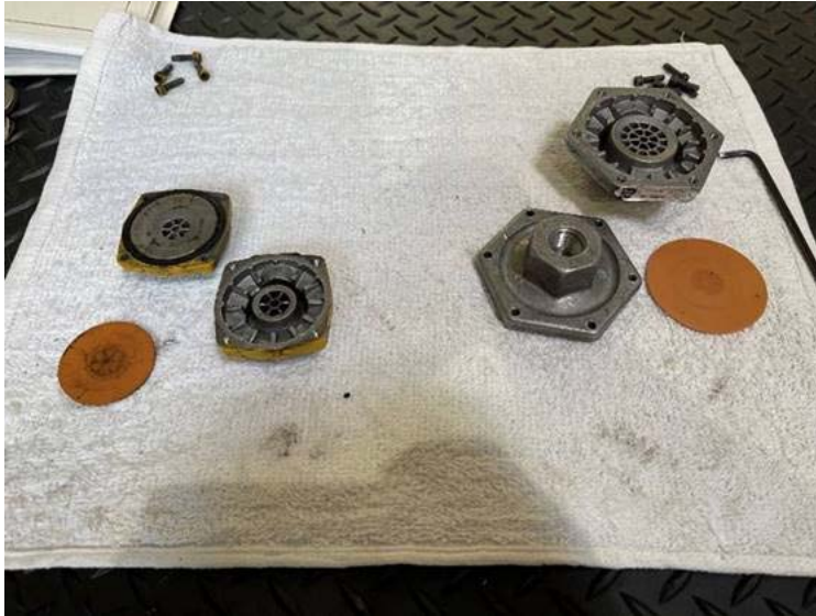
Figure 4 – PM65 Quick Exhaust Valve 77 on the left and Quick Exhaust Valve 52 on the right both replaced.
