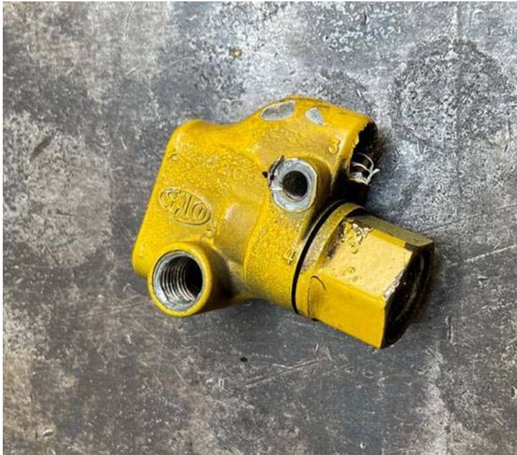
Figure 5 – PM65 Two Way Check Valve replaced.
