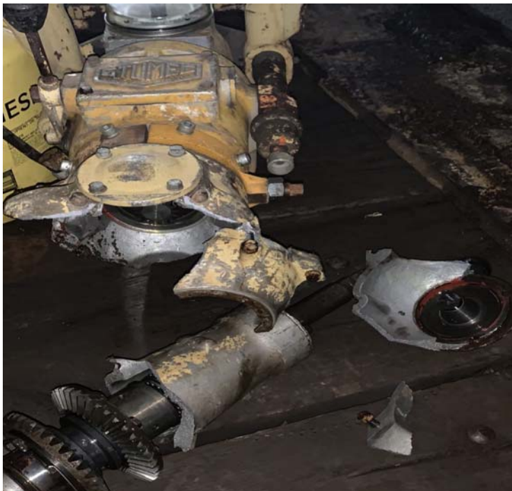
Figure 3 – Damaged Geismar Track Torquing Machine.
