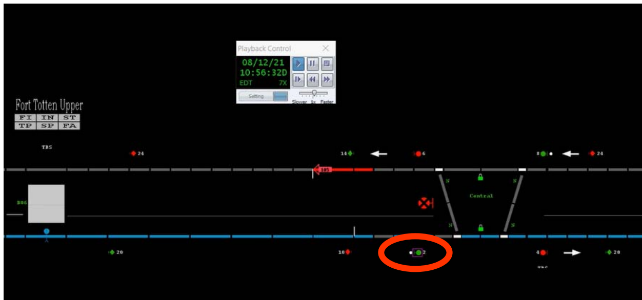
Image 1 – AIMS display after ROCC granted permission for Mobile Work Crew to enter the roadway.
