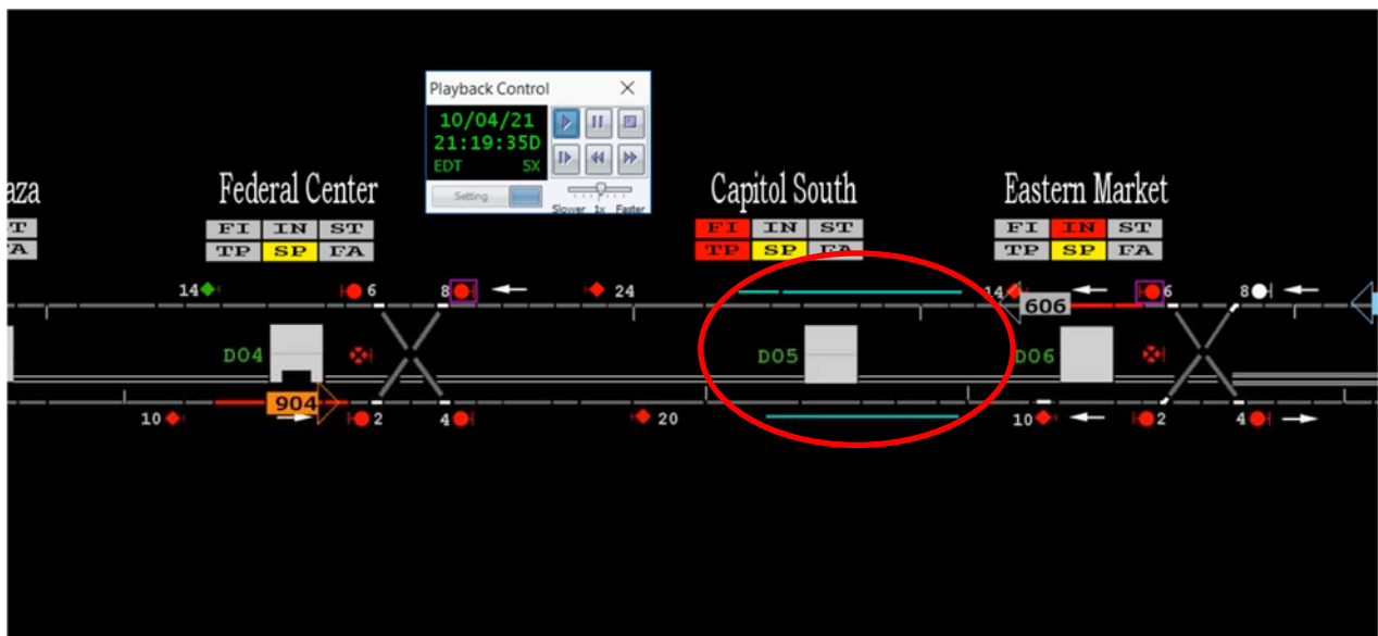
Figure 3 - ROCC commanded third rail power breakers open at approximately 21:19 hours
