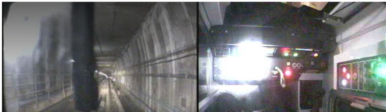
Figure 1 - Train ID 108 Train Operator attempting to take a point of power with Master Controller (MC) moved to the P4 Position.
