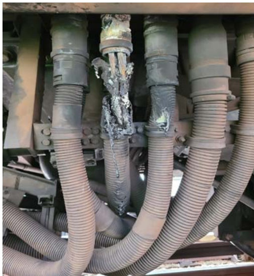
Figure 2 - Over-heated damage to cables and wires on Car 3283.
