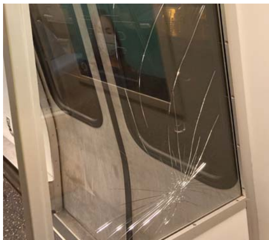
Figure 3 – Car 3040 broken interior windscreen glass.
