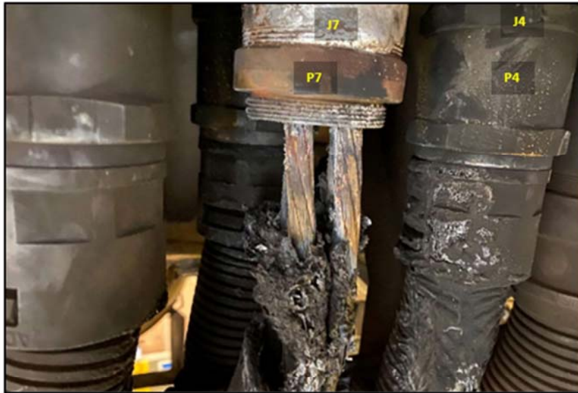
Figure 6. Damaged Connectors J7-P7 and J4-P4, Front View
