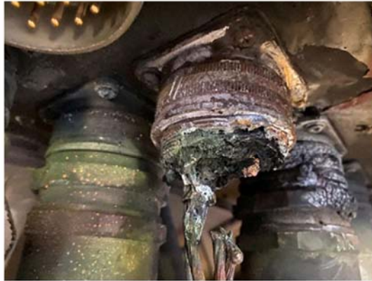
Figure 10. Rusted J7-P7 Connector
