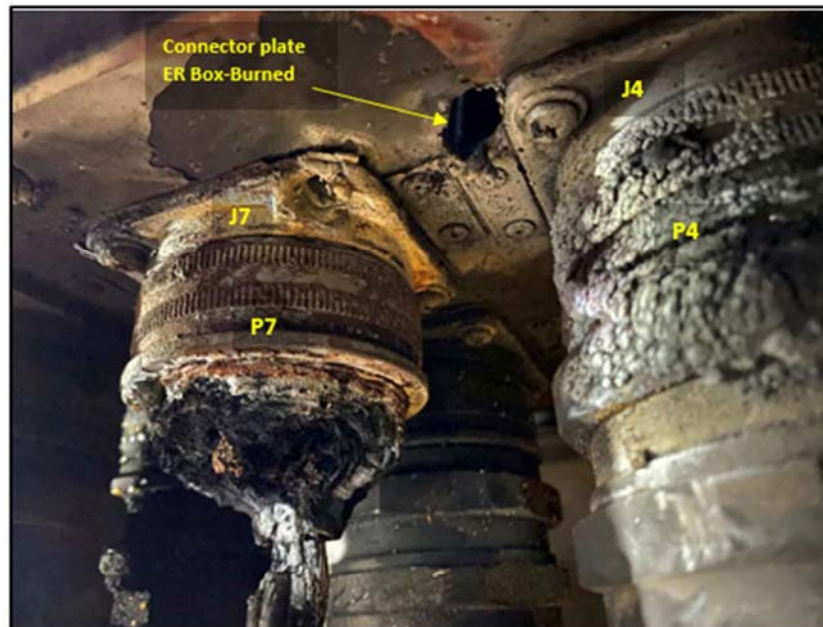
Figure 7. Burnt Connectors- View from behind
