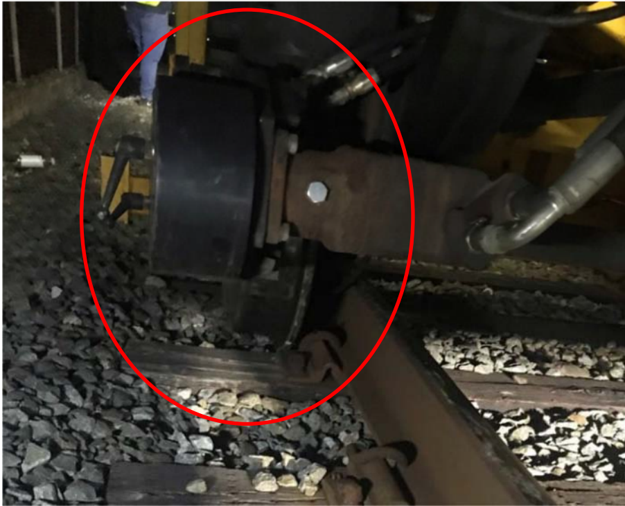
Figure 4: This image shows the front left wheel of TR05 on the ground after derailing.
