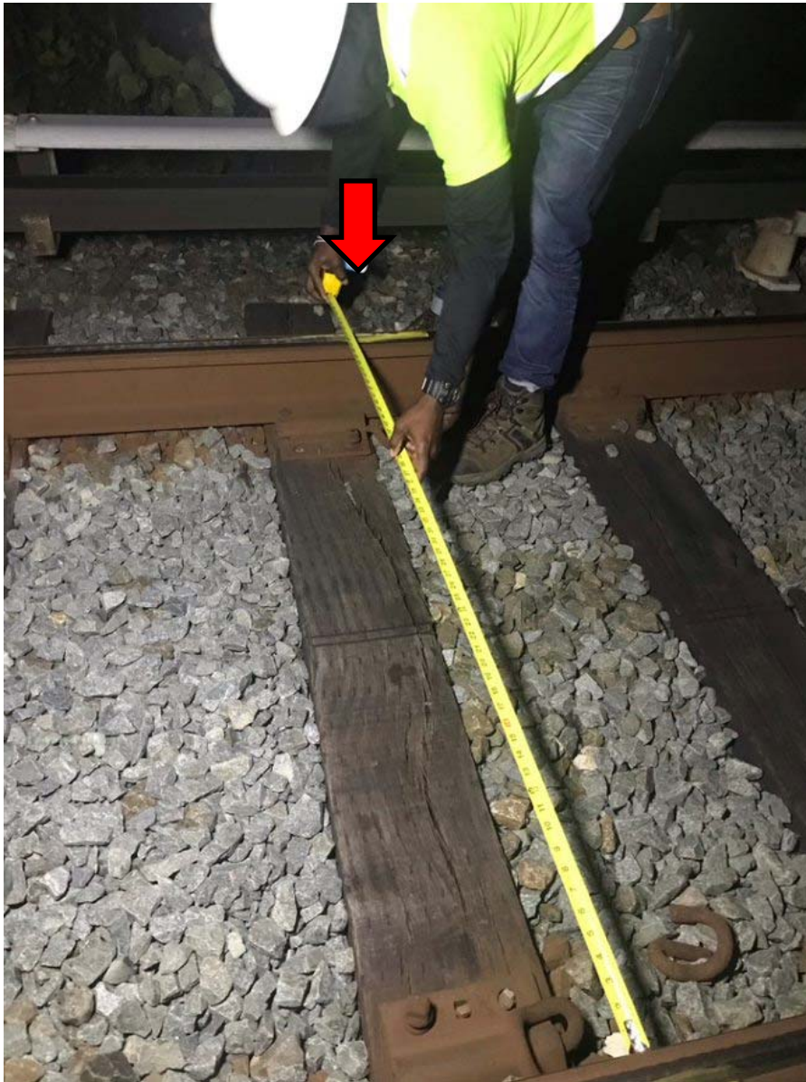
Figure 2: This image shows personnel measuring track gauge in the area of the point of derailment (POD) for TR05.
