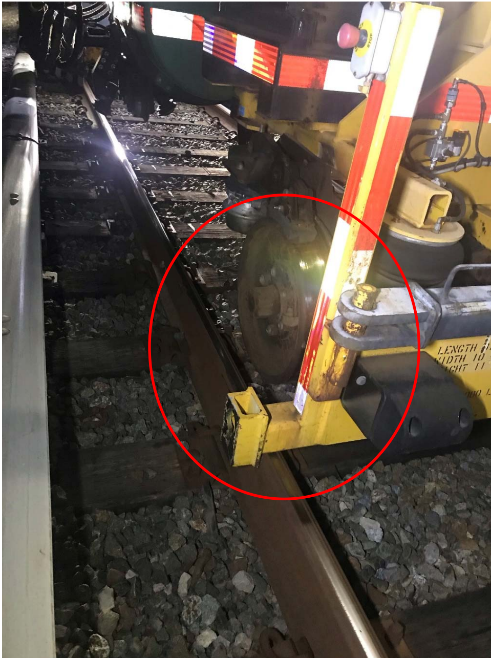
Figure 3: This image shows the place of rest of the front right wheel of TR05 after derailing.
