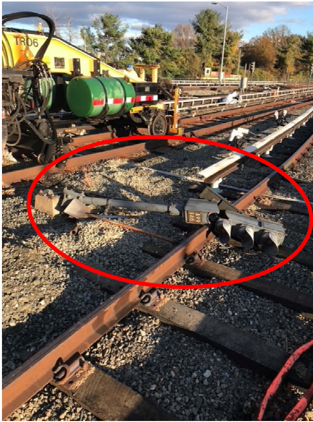
Figure 1: This image shows A99-146 signal's resting position after being hit by TR06.
