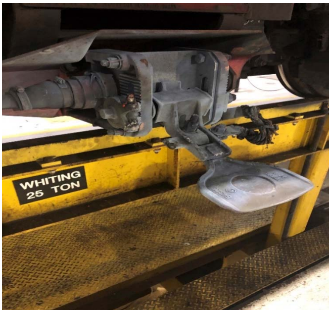
Figure 3 - Damaged rear collector assembly on Car 3105 due to the heat from the arc flash.
