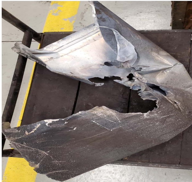
Figure 1 – The metal object that was pinned between the third rail and the right-side collector shoe on Car 3105.
