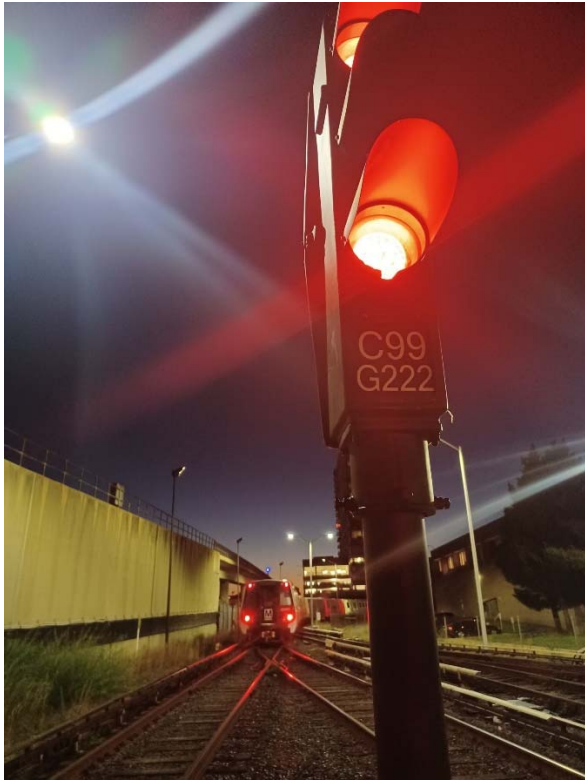
Image 2 - 4-Car Consist stopped C99-236 signal after passing C99-222 signal red and trailing switch 211.
