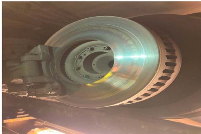
Figure 13. Worn Brake discs with evidence of heat cracks
