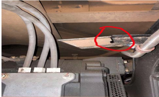
Figure 16. Rear Truck bracket broken
