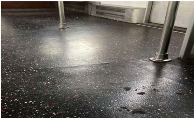
Figure 7. Car 3067 flooring deformations
