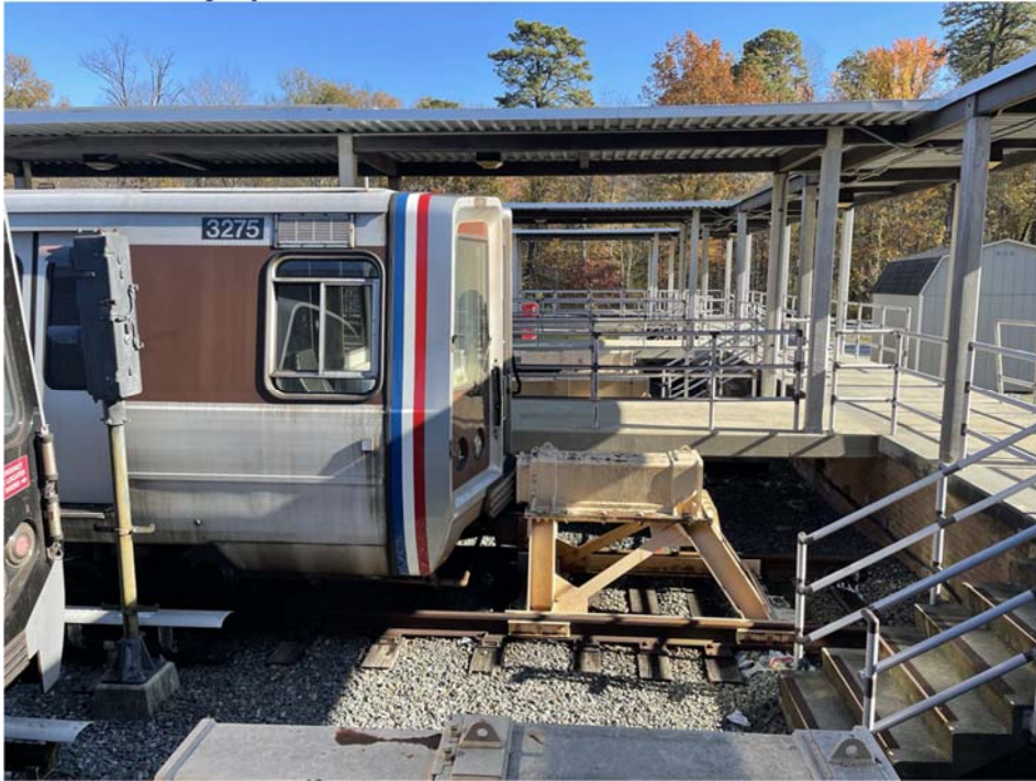
Figure 1 - Car 3275 and bump post Collision with spring-loaded barrier pushed into the housing.
