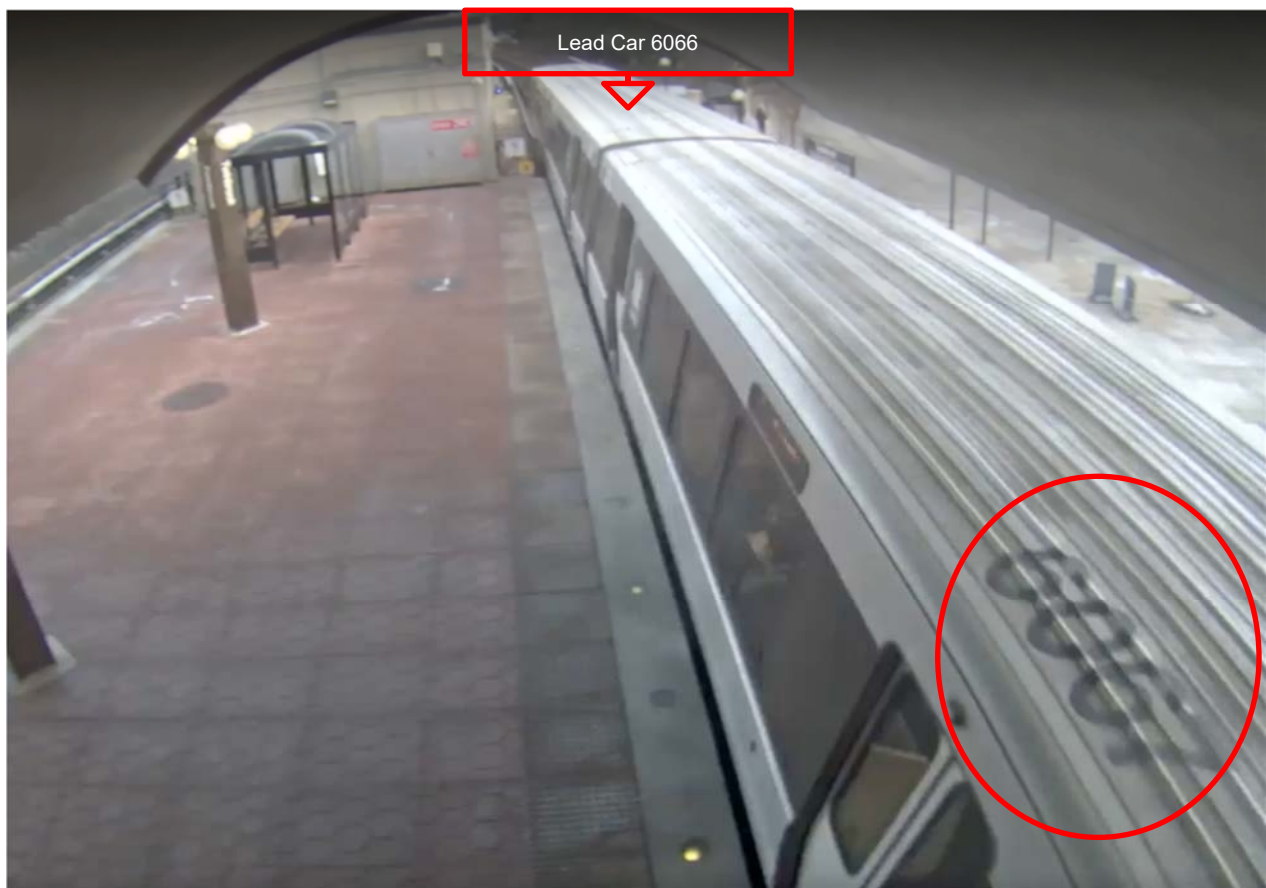
Figure 1 - Lead Car 6066 passing 8-Car Marker and continuing. This would be half of a car Station Overrun if the train stopped here.
