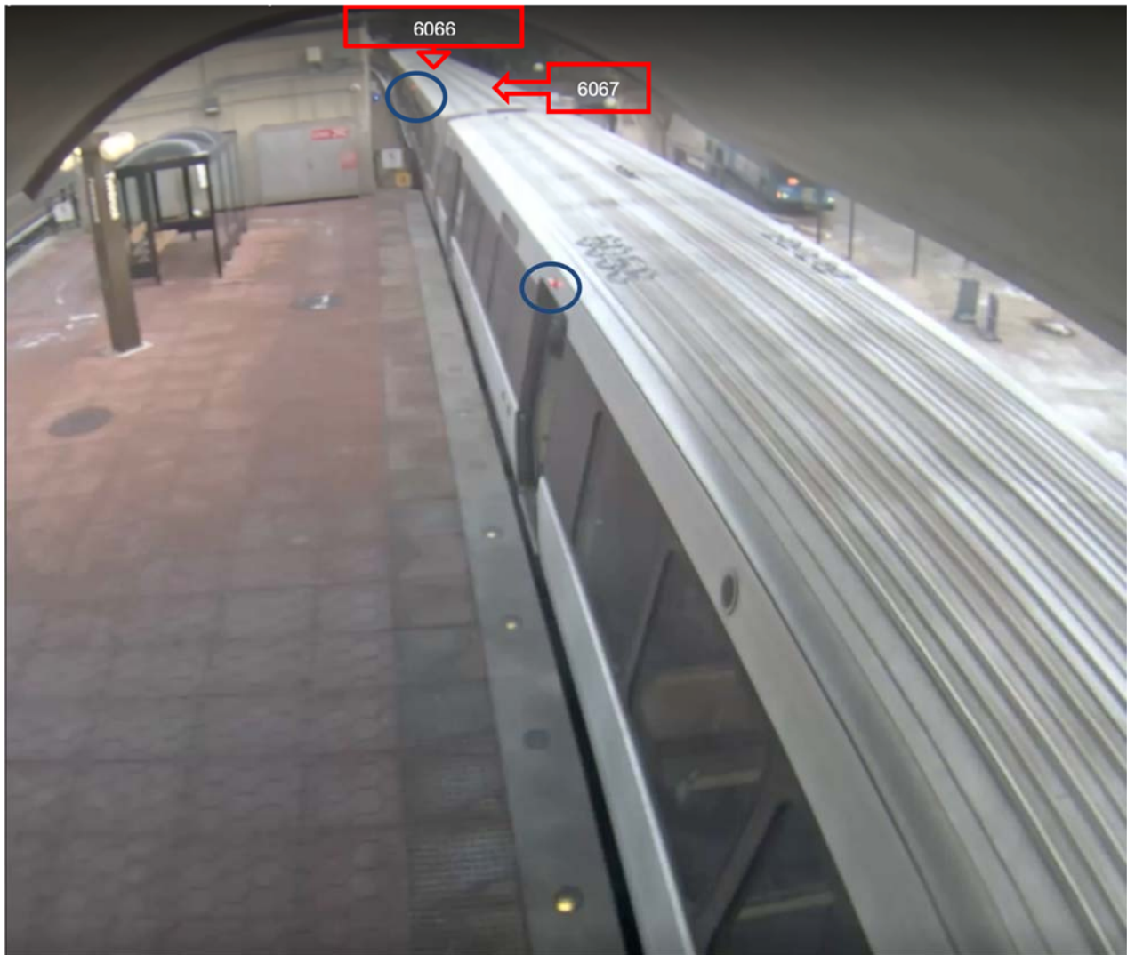
Figure 2 – Train ID 102 stopped outside of Twinbrook Station limits. Railcars 6067 and 6068’s door indication lights illuminated. 6066’s (lead car) door light did not illuminate—no platform with guard rail observed near car 6067 doors 3,4,5 and 6.
