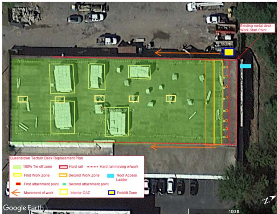
Figure 17: Diagram of Patuxent Roofing's Safety Plan and Hazard Mitigation for the site. The Arrow indicates incremental movements of 9 ft, if safe to do so.
