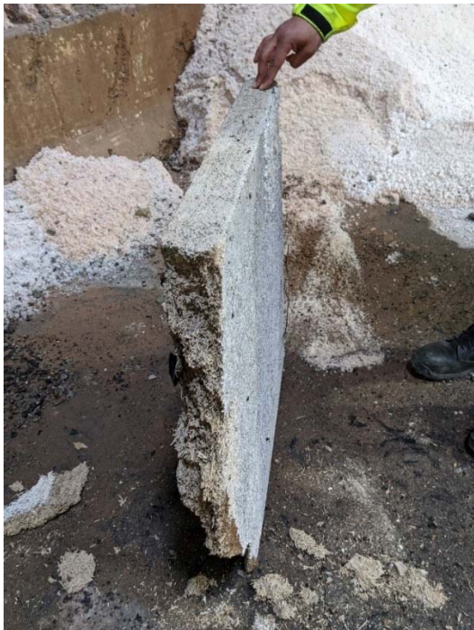
Figure 10: The largest piece of the tile with visible discoloration at the weak point. This piece was estimated to be in excess of 45 lbs.
