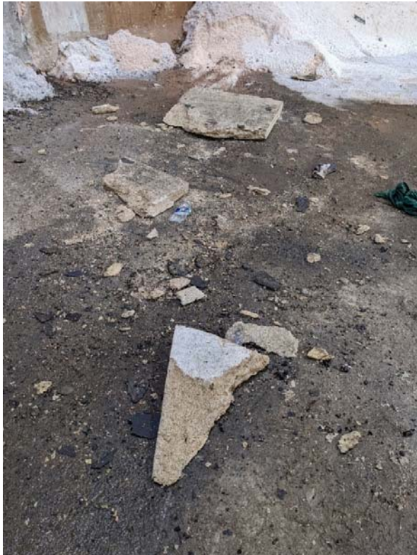
Figure 9: Close up of the shattered tile. Note the pre-existing damage.
