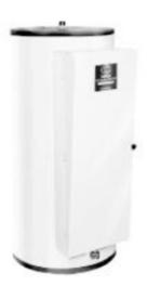
Sand blaster electric water heaters are equipped with a cold water inlet tube that directs incoming cold water to create Self-Cleaning turbulence in the tank. Self-Cleaning action keeps sediment in suspension, so it does not get a chance to settle down, and is harmlessly carried out when hot water is drawn. With reduced sediment build-up, Sandblaster retains its rated efficiency longer, lasts longer, and helps keep water heating costs down!
