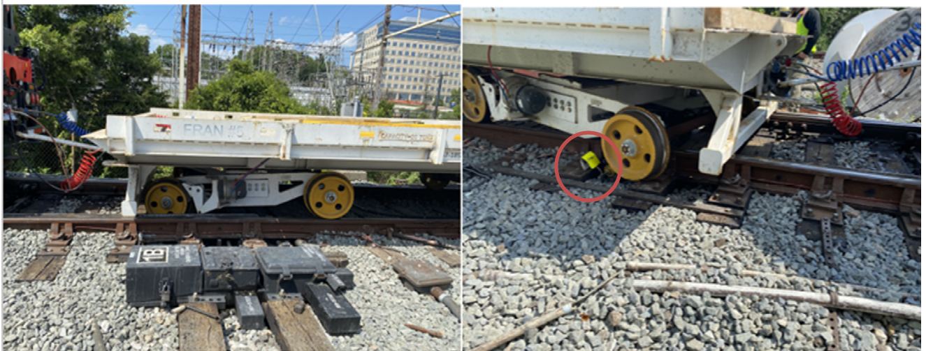
Image 2 - Kiewit Flat Car CR7719 derailed to the field side at switch 1B and Kiewit Flat Car R7719 derailed opposite the field side. Switch clamp is circled.
