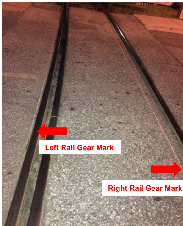
Figure 4: Shows a center view that captures the left and right rail rear gear markings.
