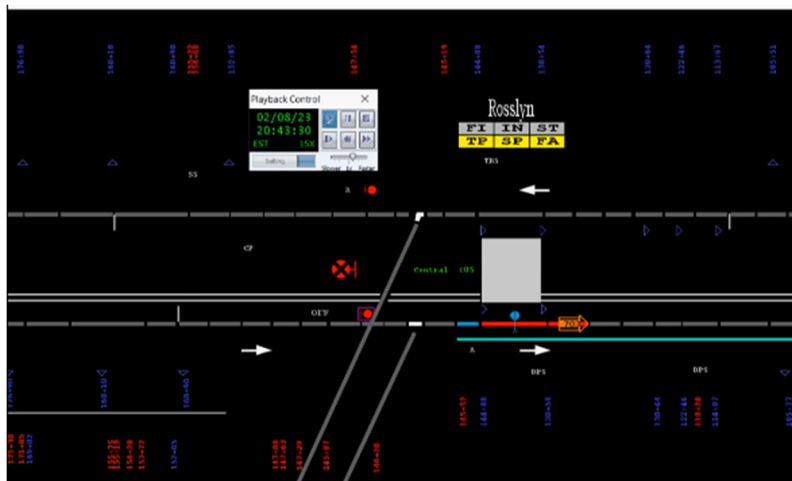
Figure 3: This image shows when third rail power was de-energized so the CMNT Road Mechanic could complete a train inspection.
