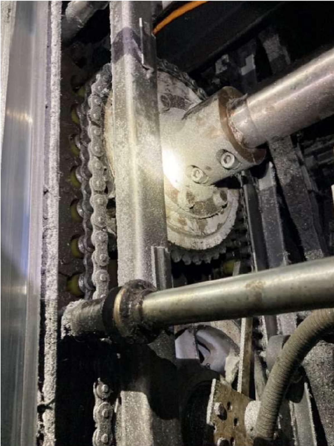
*Image 6 - Undamaged left side drive area. Notice painted finish on both sprockets.*
