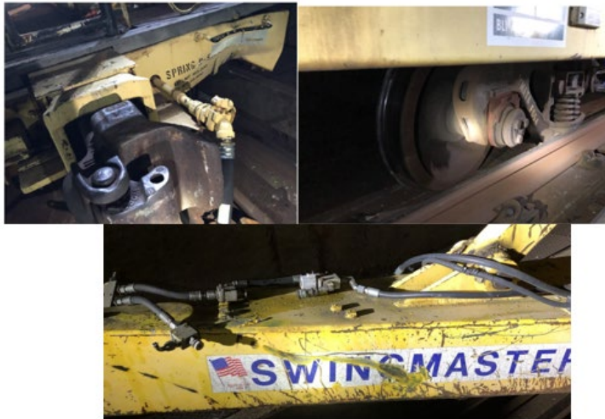
Image 2 – Photos of the damage and derailment on Flat Car 604 and SM-01 after the collision.
