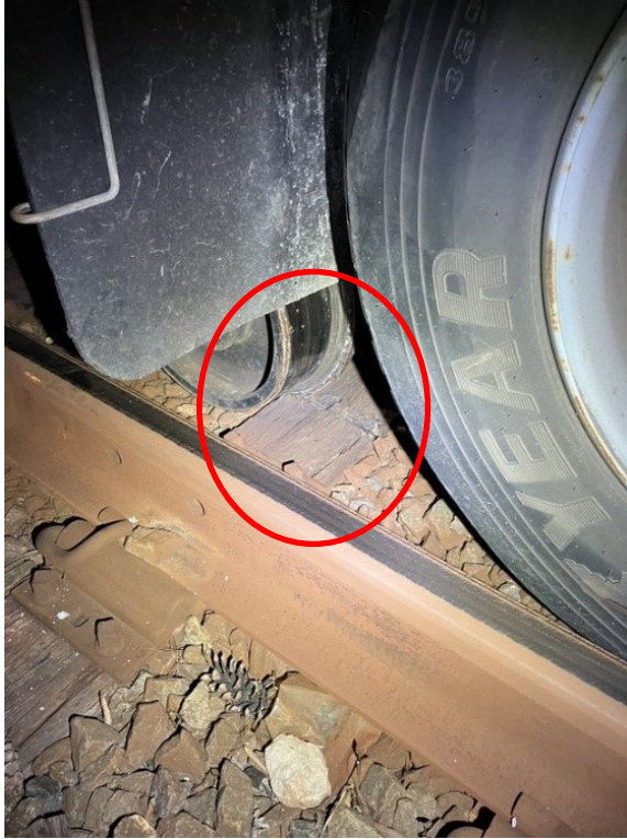
Figure 3: The shows the point of rest. Note the tie damage due to the wheel flange travel. Point of rest is approximately 26 feet from POD.
