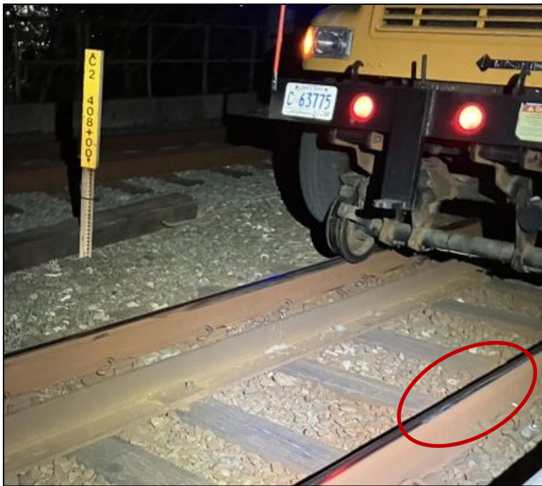
Figure 10: Point of derailment (in red), approximately two feet before Chain Marker C2 408+00. The front of the unit was the trailing end in the direction of travel.
