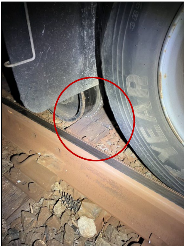
Figure 11: Shows the point of rest. Note the rail tie damage due to the wheel flange travel. Point of rest is approximately 26 feet from POD.
