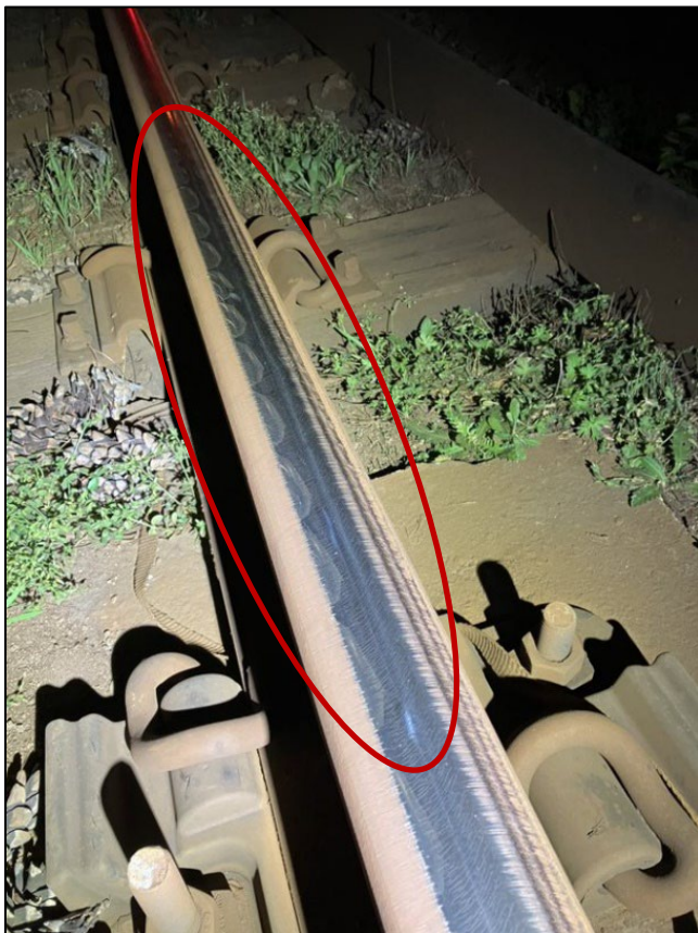
Figure 13: The rail markings switched to a swirling mark at approximately 20 feet to the point of derailment.
