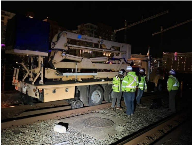
Figure 1: Hi-rail unit 14800 derailed on 04/11/23 at 01:38, travelling in reverse to Alexandria Yard along the Blue Line, between National Airport and Potomac Yard Stations.
