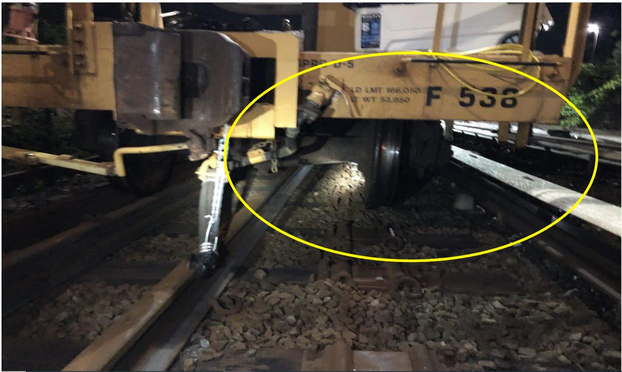
Figure 5 POR Derailed Flat Car 538. Cut sections of rail laid in the middle of the running rails.
