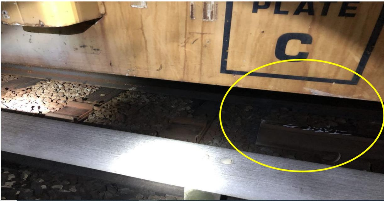
Figure 6 Point of Derailment: cut section of running rail at CM K1
