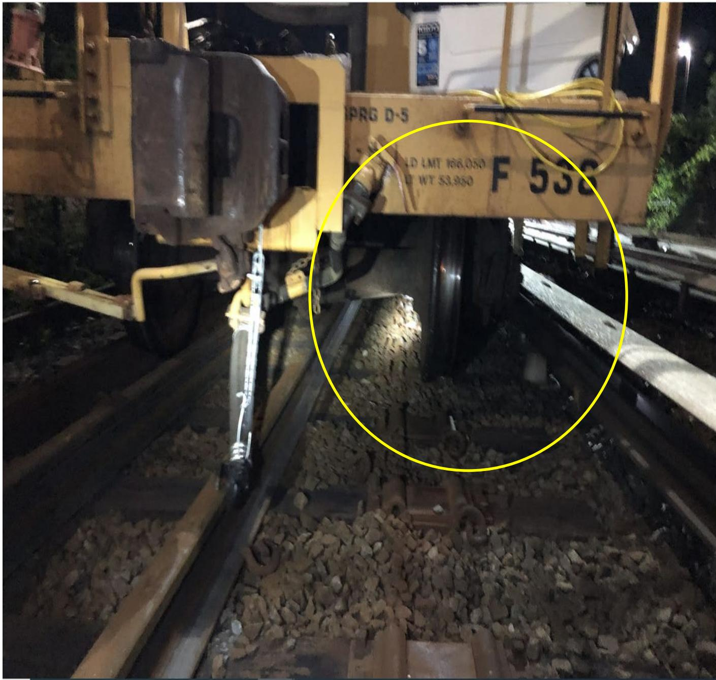
Figure 10 Flat Car 538's front wheelset (Derailment). Note the missing running rail where the rail fasteners are located.
