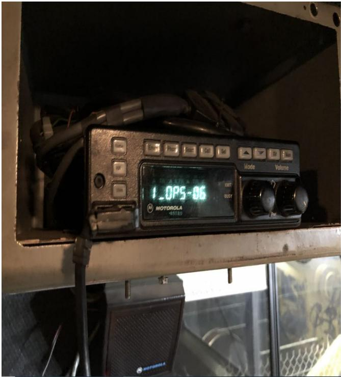
Figure 15 PM 39 radio indicates Ops 6.
