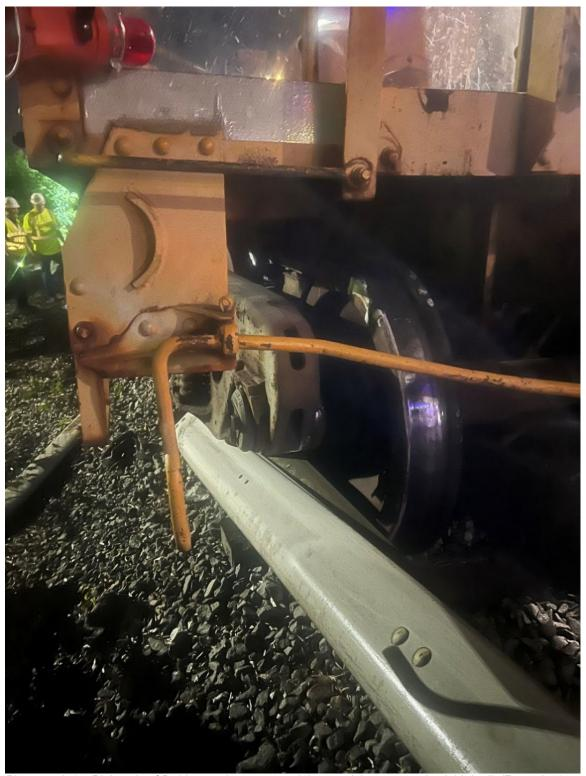
Photograph 1 – Right axle of B406 came in contact and damaged the un-energized third rail. (Front view).
