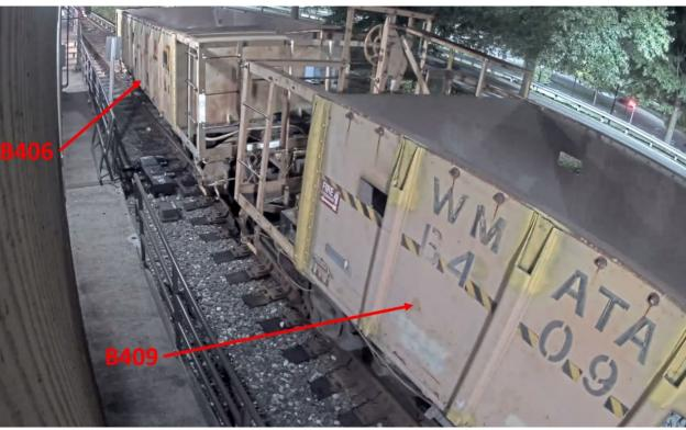
Figure 5 – Flatcar B406 with front and rear axles derailed at Switch #3A on Track 1 at approximately 00:30:39 hours.
